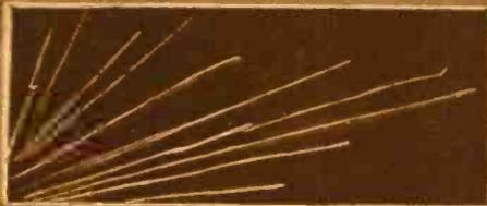
An enlarged view of the electron paths observed in the Wilson apparatus shown at top of page. Note the deviations due to the repelling force of gas atoms.
