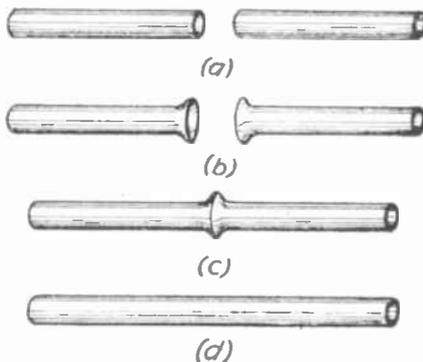
Mastering the art of glass welding will prove a very useful accomplishment of the amateur experimenter, especially in chemistry. The successive stages in the welding of two tubes of the same size are illustrated above.
