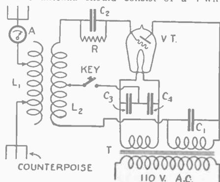
Connections of the C.W. transmitter. It may be necessary to connect a resistance across the condensers C3 and C4.
