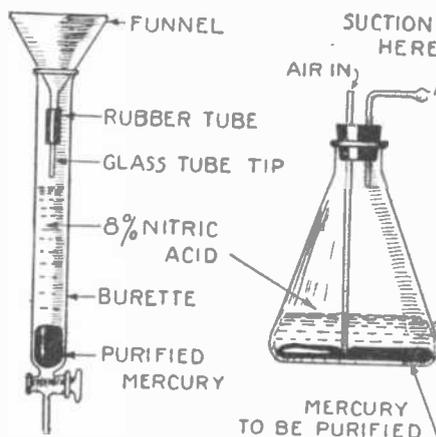
Fig. 7. The mercury used in the capillary electrometer must be chemically pure. To clean mercury either of the two methods shown above can be used. At the left drops of mercury are allowed to fall through dilute nitric acid, while at the right air bubbled through the mercury mixes the latter with the acid.
