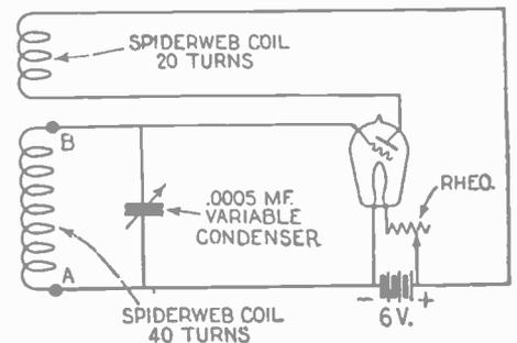
Oscillator circuit for heterodyning and laboratory measurements. No "B" battery is used.
