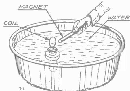
This shows the coil floating with the cork below the surface of the water and being acted upon by a bar magnet. Under this influence it performs various queer antics.
