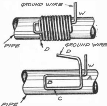
The method of making a ground connection shown above ensures a firm and extended contact surface. No sort of contact, however, can be a satisfactory substitute for a soldered one.
