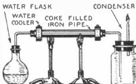
Fig. 4. Making water gas, the product of the decomposition of steam by incandescent carbon. It is a mixture of carbon monoxide and hydrogen.
