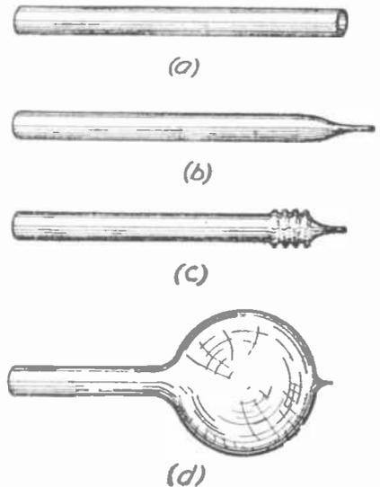
One of the more difficult problems in glass blowing is the making of bulbs out of glass tubing. First the heated glass is massed together as shown in (c), then keeping this end in the flame the operator blows into the tube, under the pressure of which air the soft glass expands.
