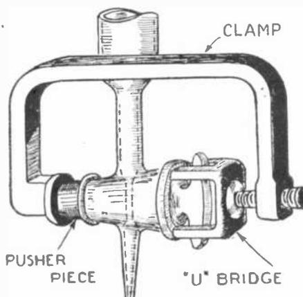
Apparatus for extracting the glass plug from stop-cocks. It is well to tap the barrel lightly with a piece of wood while applying the pressure.
