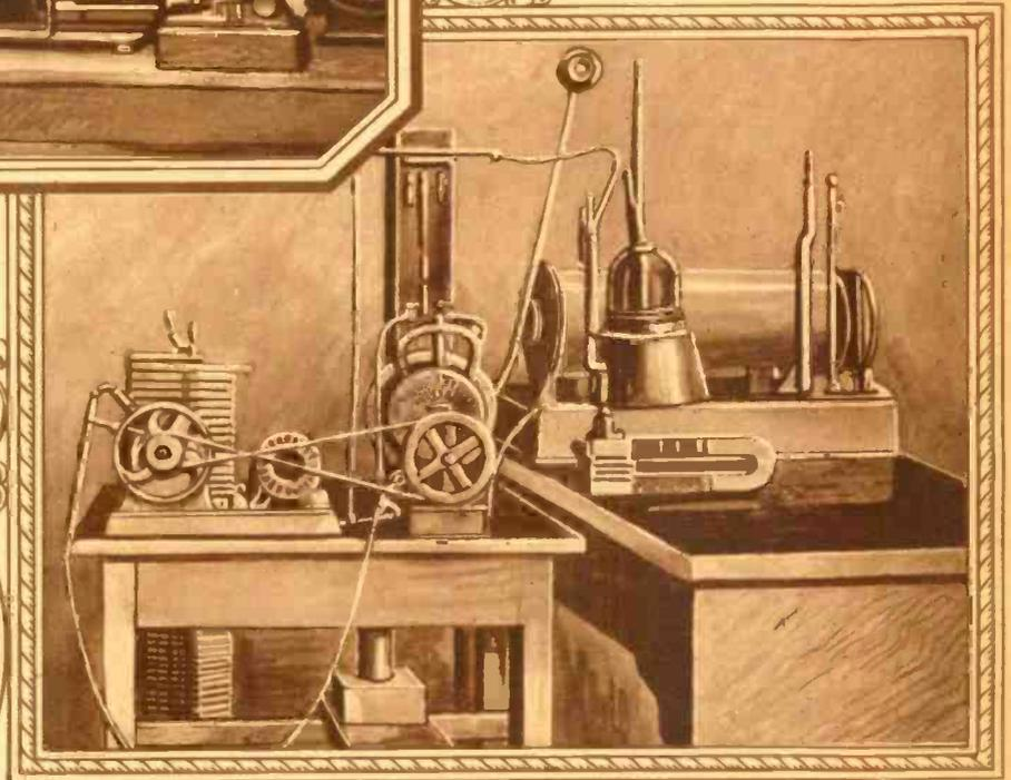
**I**ONOPLASTY is the name given to a method of depositing metals on any surface by ionic action. The diagram shows the general principle involved. (K) is the disc of the metal which is to be deposited on a non-conducting surface; the surface (L) is the one on which the metal is to be plated, which may be a plate of glass, the mirror of a reflecting telescope, or other object, and it rests upon a platinum plate carried on a base (A).
