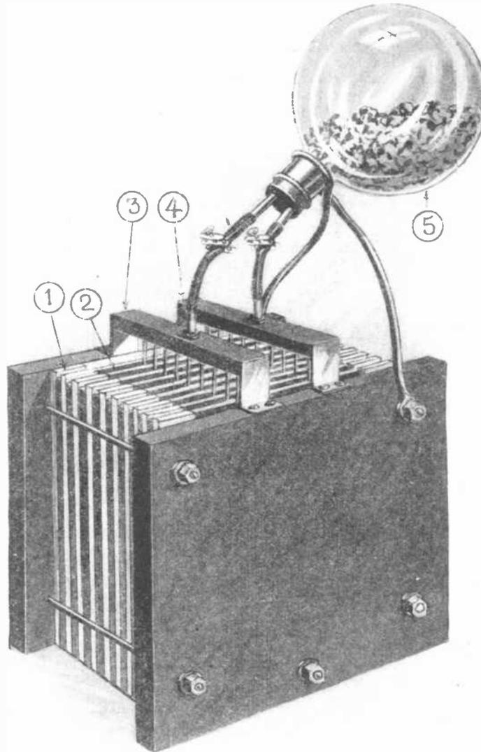
The battery above consists of a set of electrodes (2) separated by cardboard separators (1) forming small cells between the plates. From the flask (5) copper sulphate is supplied to the battery through the feeders (3) and zinc sulphate solution formed in the battery is returned to the flask through the return tube (4).
