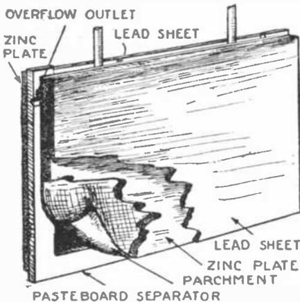
The structure of one cell of the circulation battery is shown above. As seen, each cell has a lead and a zinc electrode, the latter being covered by a strip of parchment.
