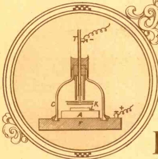
This diagrammatic view of the ionoplasty apparatus shows the plate K which emits the metallic ions which are deposited on the glass plate L as they move towards the anode F.
