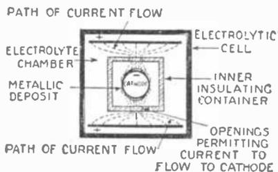
Within the bath used for electroplating there is a chamber of insulating material, within which the cathode is suspended. The insulating chamber is pierced with holes. Each one opposite to any place on the cathode it is desired to thicken by depositing metal thereon. By this apparatus local plating can be done, weak spots can be thickened, or especially thick spots can be formed on the cathode, all according to the arrangement of insulating case with its perforations.
