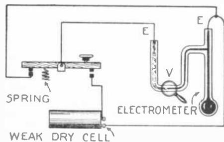
Fig. 5. The capillary electrometer is here hooked-up for demonstration purposes. The electrometer is normally short-circuited and when the key is depressed the motion of the mercury will be noticed.
