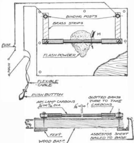
A very simple flashlamp can be constructed of two carbon pencils such as used in small arc lamps. With a gap of about 1/16" between the carbon ends a small arc between the carbons ignites the flash powder the instant the carbons are connected to a source of potential of more than 60 volts.
