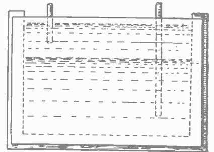
In operation, the zinc sulphate, formed by the reaction of zinc with the copper sulphate solution, rises to the top of the cell because its density is lower than that of the copper sulphate solution.
