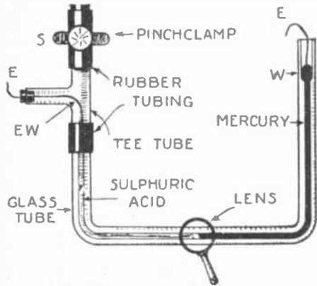
cause the movement of the mercury thread in the small bore tube. The right hand electrode (E) makes connection with the mercury, the left hand one with the dilute sulphuric acid, which of course is contained in the tube and meets the mercury at V.
