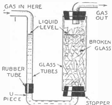
Fig. 6. Washing or absorption apparatus for gases. The large tube is filled with broken glass and the gas to be purified or absorbed is forced through it. This requires considerable pressure, but the action will be very good. Beads or glass marbles may be used instead of broken glass.
