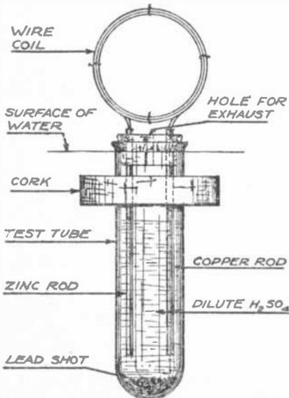
A very small battery is arranged in a test tube ballasted with lead shot and buoyed up by a cork. The cork is completely submerged and the current through the coil gives a number of interesting experiments.
