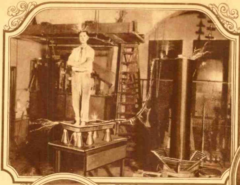
The man above is taking a 40 kw. high frequency discharge from the Tesla coil at the University of California. The coil used in these experiments is seven feet high. The current passes over the surface of the body only.
