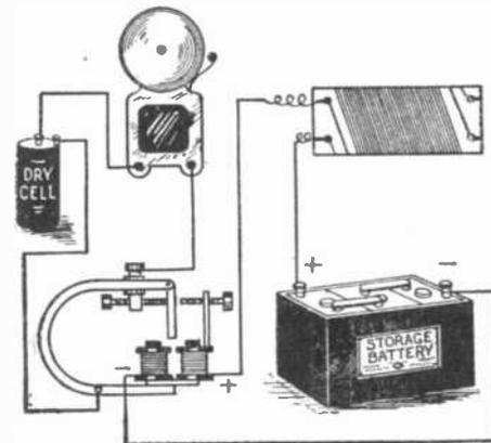
A common application of the selenium is shown above. The cell under the influence of light will have a reduced resistance and allow the passage of sufficient current to actuate the relay, which in turn closes the bell circuit.
