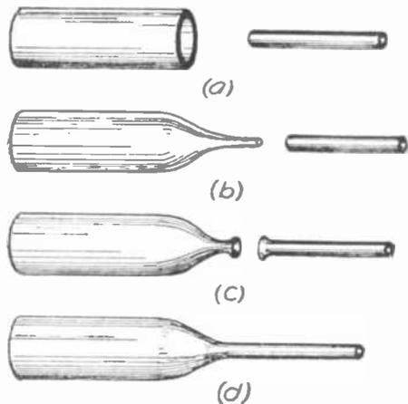
In welding two tubes of unequal sizes, the end of the larger must first be drawn and tapered down to the diameter of the smaller. The operation is shown in three steps.
