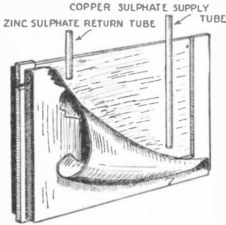
The illustration shows the disposition of supply and return tubes in each cell. The copper sulphate tube conducting the heavier solution reaches to the bottom of the cell.
