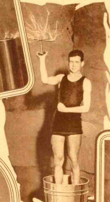
The sparks emitted by the arms of the small rotor at the left impart to it a spectacular motion. The Tesla coil is connected to the salt water bath in which the man stands.
