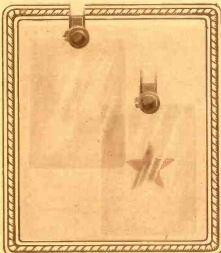
The glass plate at the left has been exposed for five seconds, the central area being screened by a star-shaped plate, to an ionoplasty of silver. The faint deposit was invisible until it was amalgamated by exposure of mercury vapor, producing the effect shown at the right.
