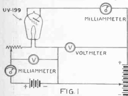
Method of connecting the meters, batteries, and tube for plotting the characteristic curve shown in Fig. 2.
