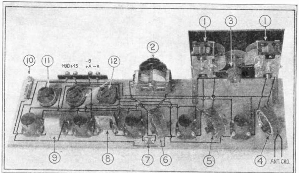
Fig. 7. An experimental five-tube receiver in which two of the tuned circuits are controlled by one dial. The condensers (1) are geared to one dial. The condenser (2) is controlled separately. (3) is a small vernier condenser for fine adjustments. (4), (5) and (6) are the low loss coils. (7) is the grid condenser and leak. (8) and (9) are audio transformers. (10) is the jack, (11) the six-ohm rheostat and (12) the 30-ohm rheostats.
