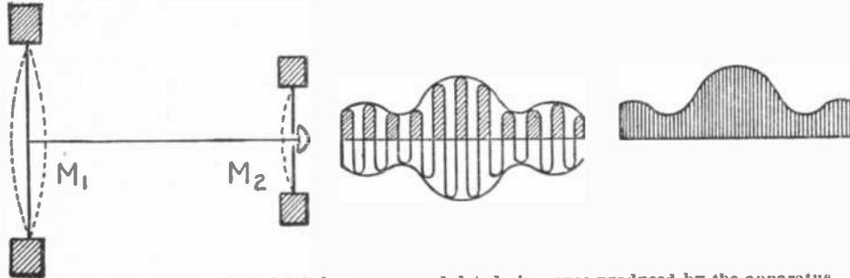
Fig. 2, the receiver of the high frequency modulated air waves produced by the apparatus shown in Fig. 1. Note that diaphragm M2 is actuated upon by only one-half of the incoming wave, giving the effect analogous to rectification or detection.
