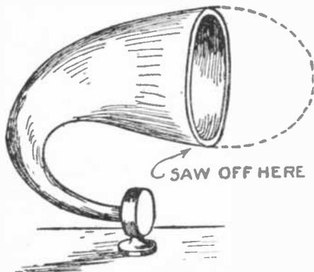
By sawing off the end of the gourd, its acoustic properties are improved. The tone is very mellow and does not have the harshness so common to metal horns.
