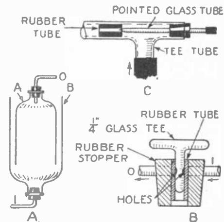
Fig. 8. Outline of a gasometer and two more versions of stop-cocks for use in gas experiments.
