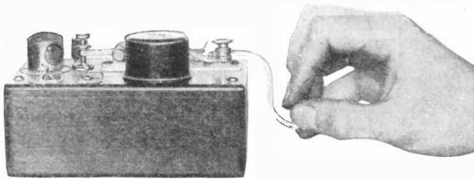
Fig. 3. The correct position for holding a telegraph key when transmitting code. Note that the entire arm and not the fingers should be used for operating the key.
