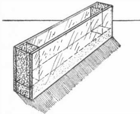
A lantern demonstration cell such as that illustrated above can be readily constructed by the experimenter who acquaints himself with the simple methods of glass grinding and cementing.
