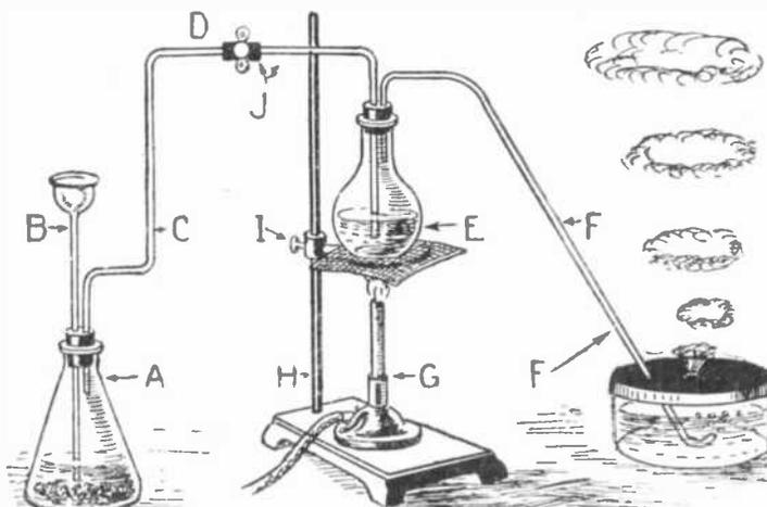
Generation of phosphoretted hydrogen or phosphine; this gas when thus generated is not absolutely pure and there is enough of another hydride in it to make the mixture spontaneously inflammable, as the pure gas,  $\text{PH}_3$ , does not possess this property. Beautiful smoke rings are produced as bubble after bubble ignites.
