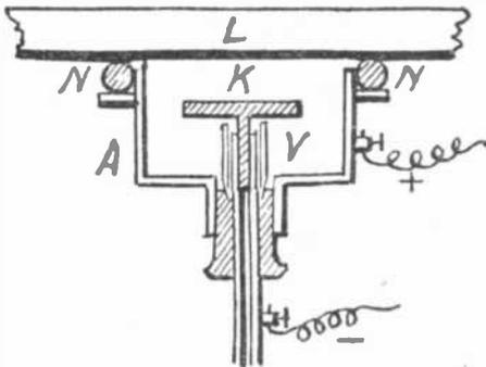
A modified form of ionoplasty apparatus is shown above. The glass bell jar of the previous type is here replaced by a metal case. This form was specially designed for coating large telescope mirrors with silver film.
