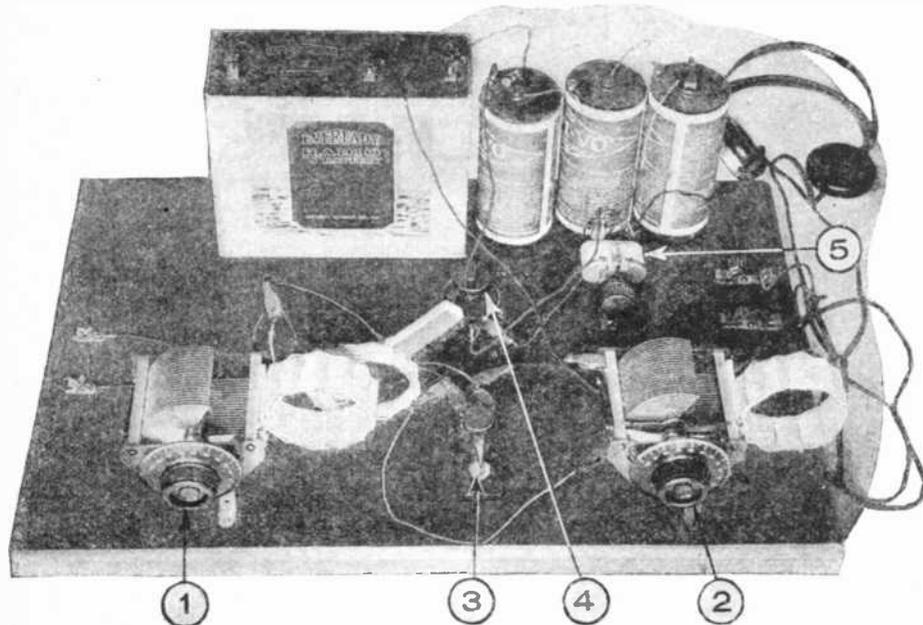
Apparatus used for making experiments with oscillating crystals—1 and 2 are tuning condensers on which are mounted the low loss coils; 3 is the zincite crystal detector; 4 is the potentiometer and 5 the variable resistance.
