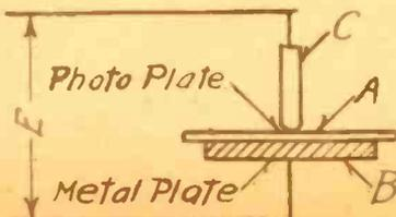
**A** NEW instrument, known as the klydonograph, has been developed by J. F. Peters, of the Westinghouse Electric & Manufacturing Company, for recording abnormal voltages on transmission lines. With this instrument, a graphic record of voltage surges of extremely short duration can be obtained, giving their polarity, magnitude, steepness of application, etc.
