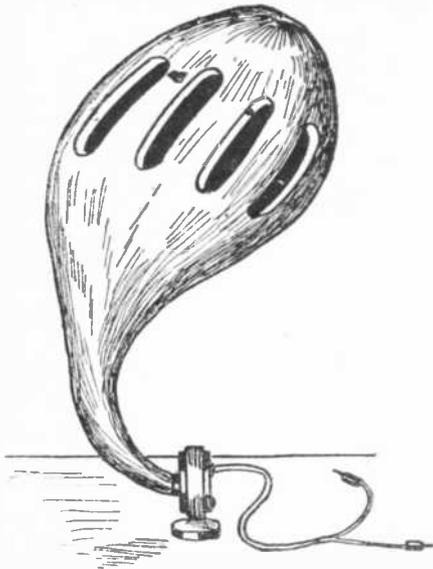
Showing how a common gourd, after it has become hard and the seeds are withdrawn, is used as a loud speaker horn. Note the slots in the sides through which the sound waves pass.
