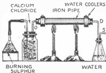
Fig. 5. The same apparatus slightly modified for manufacturing sulphuric acid. The iron pipe contains catalytic ferric oxide, which effects the oxydation of the sulphurous oxide.
