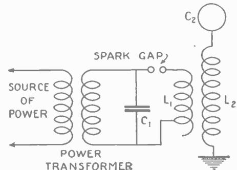
The diagram illustrates the connection of the Tesla coil to a power transformer. A condenser C1 is constructed of a large number of milk bottles containing salt water, themselves immersed in a large pan of salt solution.
