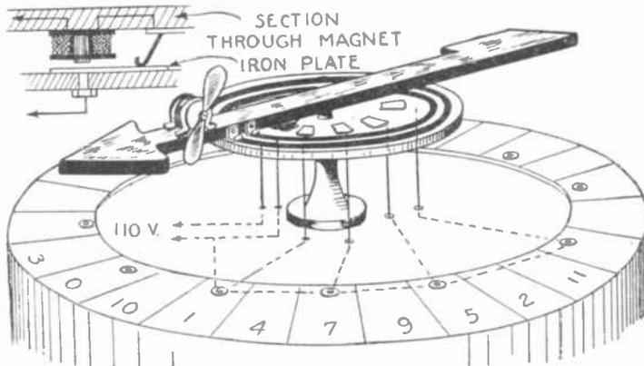
This game is extremely simple and the electric motor is used merely to start the arrow spinning. The switch open, the arrow is allowed to come to rest, the prize winning number being indicated by the arrow.
