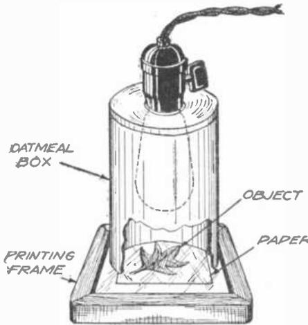
An oatmeal box with one end removed is here furnished with an incandescent bulb and used for blueprinting on cloudy days or at night.
