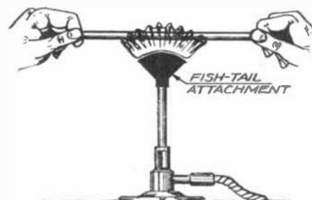
Glass bending is one of the easiest operations met by the glass worker. Good glass tubing becomes very pliable and easily worked when heated to the proper temperature.
