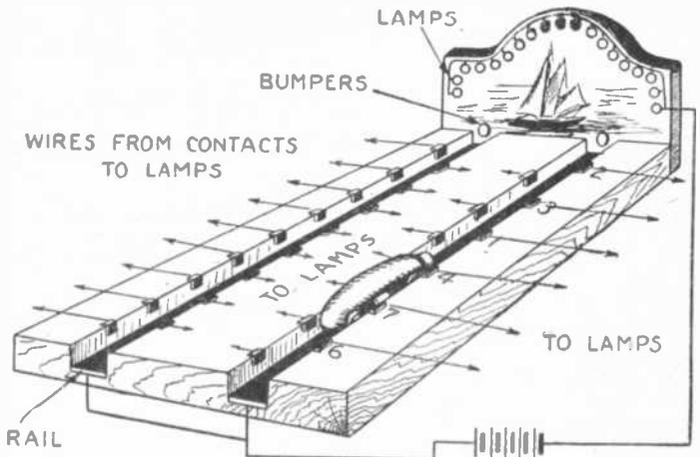
This is another game built on a war motive. Rolling over a conducting rail to which one terminal of the battery is connected, the steel torpedo as it is pushed forward and rebounds from the bumpers, makes successive contacts with segments connected to numbered lamps. The lamp which remains lit after the torpedo stops announces the lucky number.
