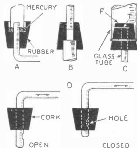
Fig. 7. Extemporized valves and stop-cocks employing rubber stoppers and glass tubing only.
