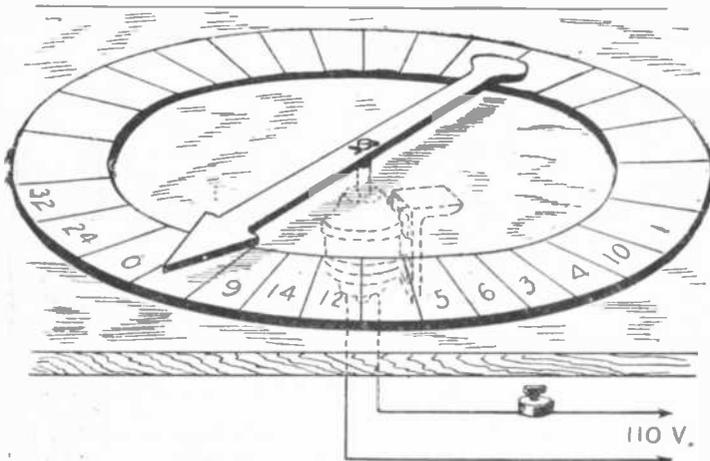
A large wooden arrow rotated by the action of an electrically driven propeller carries a brush and an electromagnet on its underside. The brush and the magnet move over iron segments. Each player has his own switch which he tries to close at the instant the magnet passes over the corresponding segment. When this succeeds the attraction between the magnet and the iron segment will cause the arrow to stop and point to the winning number.
