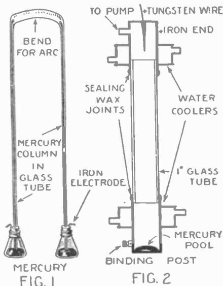
The mercury vapor lamp of Fig. 1 needs no pump to evacuate it. The tubes made slightly more than thirty inches long are filled with mercury. When the tubes are inverted and placed in operating position the mercury level drops, leaving a perfect vacuum at the top. Fig. 2 shows a form of lamp which requires no glass blowing. Iron caps are sealed to the ends of a glass tube. The joints are water cooled.
