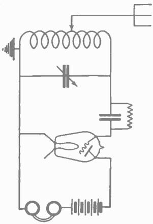
The idea which this data sheet is intended to emphasize is the fact that the electron tube always operates the same, no matter in what kind of electrical circuit it is used. It always has its input and its output circuits, the weak incoming signals being fed into the input or grid-filament side, and the strengthened signals coming out of the output or plate-filament side.
