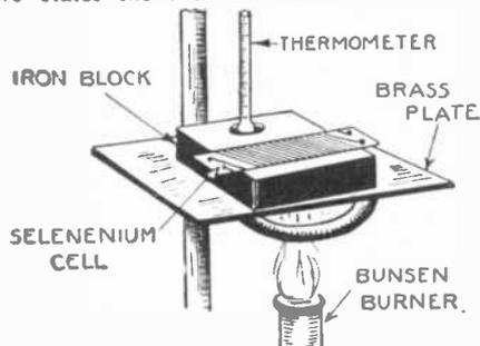
Powdered metallic selenium is melted on the sheet of mica or slate on which copper or iron wire has been wound as shown above. The melted selenium fills the space between the wires and when allowed to cool, crystallizes.
