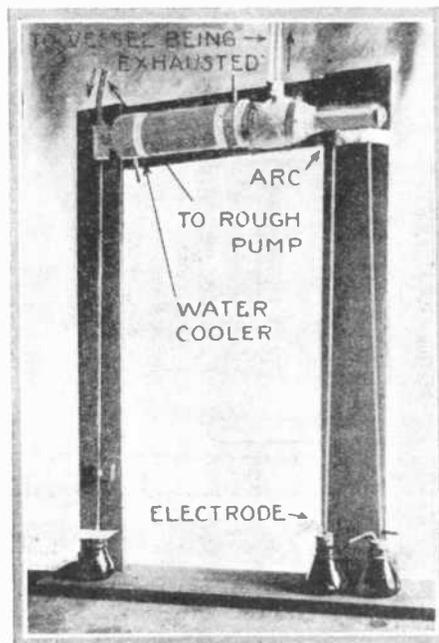
By connecting the mercury vapor lamp consisting of the two tubes at the right to a condensation chamber at the left an efficient low pressure pump is formed. The mercury vapor passing out of the arc draws gas molecules with it and thus evacuates the chamber to which the apparatus is connected.
