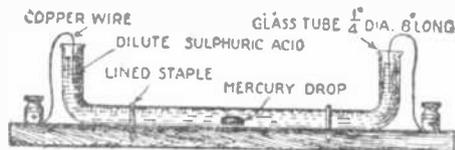
The principle of the capillary electrometer illustrated by a home-made appliance; a most interesting piece of apparatus, depending for its action probably on surface tension of liquid mercury.
