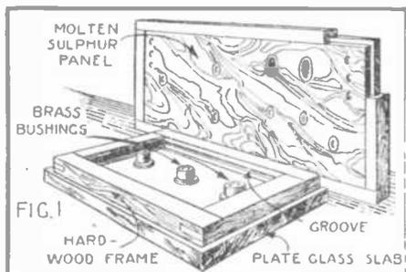
An attractive panel for your radio set can be made from cast sulphur, requiring very little machining after the cast has cooled and is withdrawn. Screws and bushings can be imbedded in the hot sulphur, enabling the experimenter to construct his panels in a very short time.
