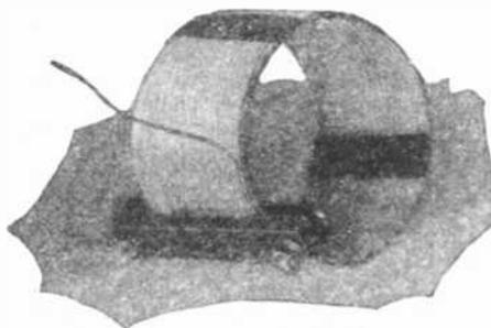
Another form of low loss coil which the experimenter can easily wind. It is self-supporting except for two strips of gummed paper and the hard rubber clamps.
