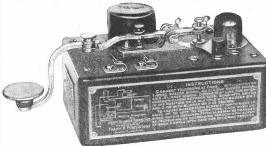
Fig. 2. A code practice set used by the army. This comprises key, buzzer, batteries and a small signal light.
