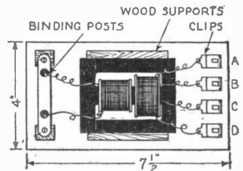
Top view of the assembled shell type transformer. While the figure shows no clamps, it is important that some means for clamping the laminations be used.
