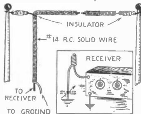
Static may be reduced by winding an insulated wire on the entire length of the aerial and grounding it.
