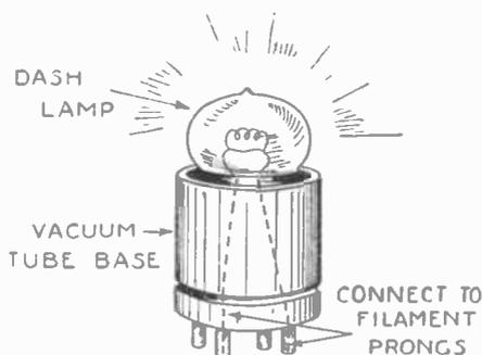
A dash lamp fitted into the base of a vacuum tube for testing the wiring of radio sets.
