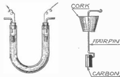
On the left is shown a simple U-tube with double perforated corks which will take the place of the expensive one shown in the other illustration. The way the carbon electrode is immersed in the solution and supported is shown on the right hand.
