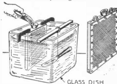
This is a cell with sides of perforated insulating material such as celluloid; there is a hopper which leads into the interior and in use it is to be filled with pellets or lumps of the metal to be deposited. As long as there are pellets of metal in the funnel, a circuit is completed through the metal of the hopper and the two suspending lugs, one on each side of it, and the top plate of the cell to which all three are secured.
