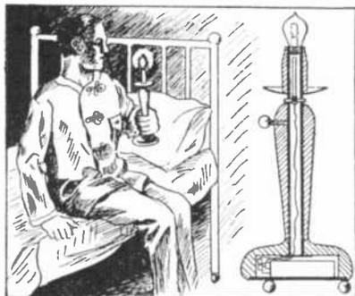
The lamp is supported on the end of a metal tube. Near the top of the tube there is a vertical rod which is free to move up and down and a transverse bar at the foot of the rod projects through slots at the side of the tube. When the lamp is taken up in the hand, an outside wooden tube which surrounds the tube slides upwards, strikes the transverse piece, pushes up the brass rod so as to touch the base of the lamp, and this completes the circuit from the supply battery contained in the base.
