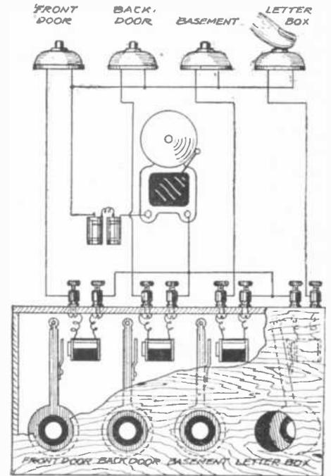
With a number of doors to a house and as many push buttons operating a single bell, what housekeeper has not been irritated by the problem of determining at which door the button was pushed? To these housekeepers the simple annunciator illustrated above will be a godsend.
