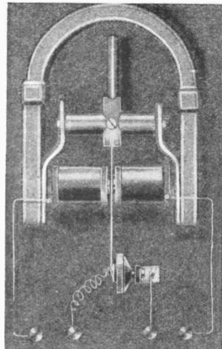
Photograph and diagram of the microphone amplifier showing how it is connected to a vacuum tube receiving set. This simple device amplifies local concerts loud enough to operate a loud speaker.
