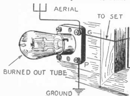
Showing how a burned out vacuum tube may be used as a radio lightning arrester.
