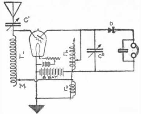
A single circuit receiver with regenerative feed-back and a crystal detector. Extreme distances have been covered with this experimental hook-up.
