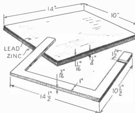
The drawing shows detail of electrodes and separators. The electrodes are double; a zinc plate about a quarter inch thick is covered on one side with the lead sheet one-sixteenth of an inch thick. One is the positive and the other is the negative plate.
