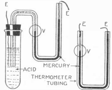
The apparatus illustrated above, Figs. 1-3, are various forms of the capillary voltmeter. The essential feature is a thin capillary tube containing sulphuric acid and mercury, each in contact with one terminal of the source whose potential is to be measured. The passage of a minute electric current alters the surface tension at the boundary between the mercury and sulphuric acid and causes the thin mercury stream to move. This motion is observed with a lens or microscope.
