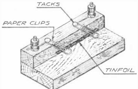
With two paper clips some little wooden blocks and a bit of tin foil or thin wire, the young experimenter constructs a fuse to take care of his work without disturbing the fuses (and the family) on the house circuit.
