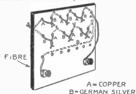
The illustration shows the manner in which the thermo couples of a thermo-battery are connected. The couples are connected in series as the potential difference in a single couple is slight.
