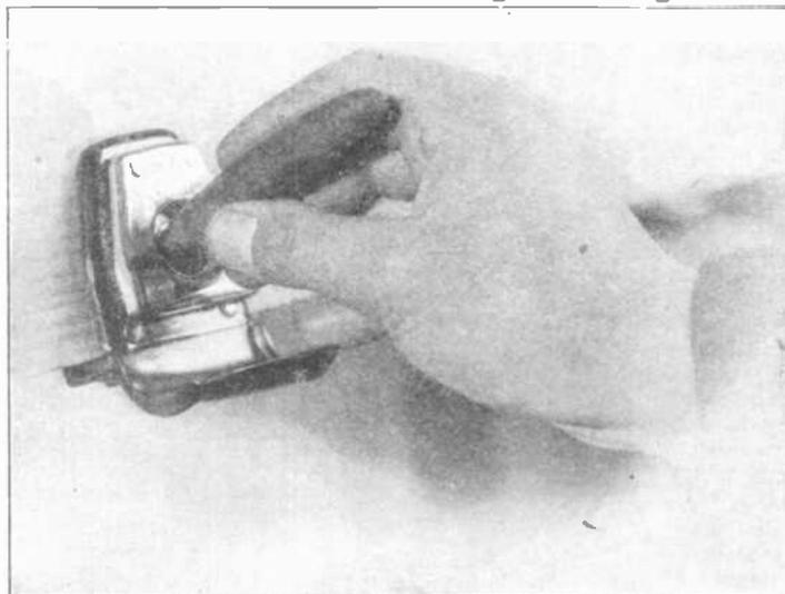
The cigar-lighter carried on the dash-board of a car has a lid, which is closed. The closing opens the circuit. To light a cigar the lid is dropped which closes the circuit and the heating element becomes red hot and will light a cigar in a few seconds.
