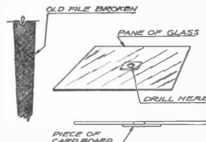
No special apparatus or very great skill is required to drill holes in plate glass. An old flat triangular or round file sharpened to a point, some turpentine as lubricant, and a little care, are the essential requirements. Note the little piece of cardboard.
