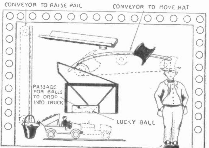
The diagram shows the operation of the "Candy Kid" game. The conveyor at the left lifts the pail of balls and tips them into the channel at the top. At the same moment the conveyor at the right carries the silk hat under the opening of this channel. Having received the balls the hat is carried by the conveyor to the hopper into which the balls are tipped.
