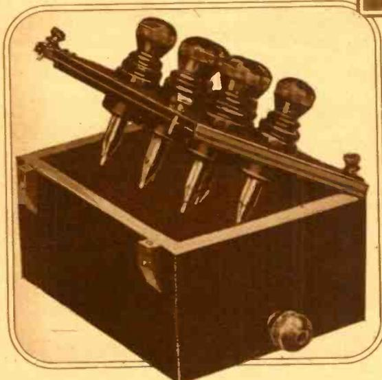
The diagram shows the operation of the klydonograph. Between the electrodes B and C the photographic plate A is placed. The corona discharge occurring between the two electrodes is recorded on the plate.
