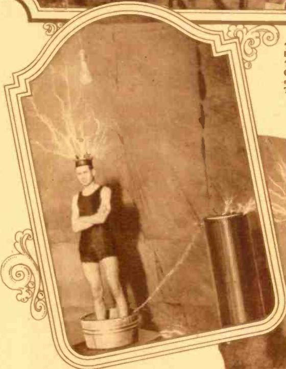
The discharge above is radiated from a metal crown worn on the head. The use of this crown eliminates the danger of burning the hair.
