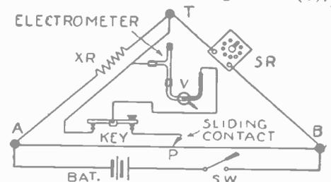
Fig. 6. The capillary mercury electrometer will serve as a useful current indicating device in connection with a Wheatstone bridge. Note that the electrometer must normally be short-circuited.
