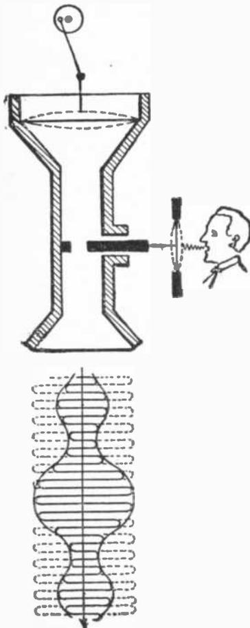
Fig. 1. Showing how high frequency air waves produced by the machine at the top are modulated by low frequency voice waves. The resultant wave shape is indicated at the bottom of the illustration.
