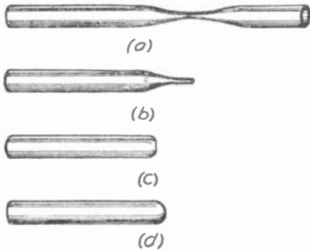
The method of making sealed glass tubing is shown above. The glass tube first tapered is then exposed to the flame long enough to cause a complete closing and rounding of the end.
