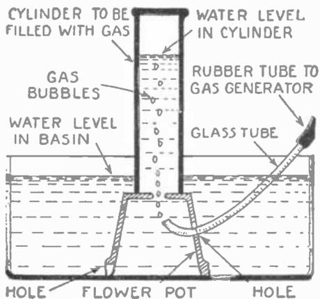
A flower pot is used to carry a vessel to be filled with gas in a hydraulic trough. The interesting feature of the flower pot is that it is so soft that it can be readily drilled to admit a tube.
