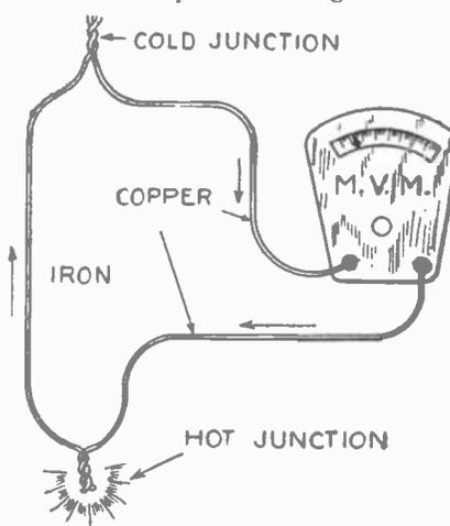
A sensitive thermo couple should have besides a hot junction a cold junction kept at a constant and known temperature. The electrical circuit of such couple is shown above.
