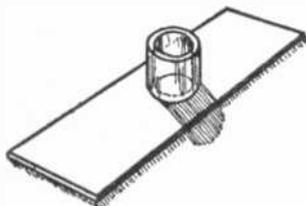
A short section of glass tube is ground off on the ends and is cemented to a microscope slide. This gives a cell for microscopic work.
