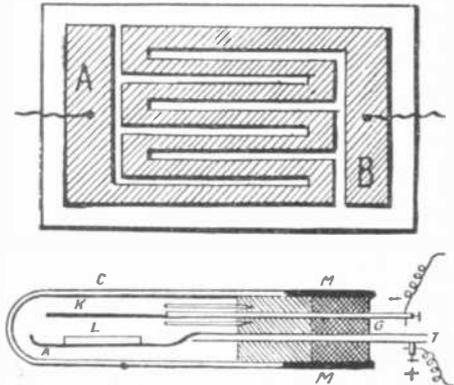
At the top is shown a very high metallic resistance consisting of a very thin film of ionoplastic silver. Such resistances are high enough to be used as grid leaks in radio, where at present metals are rarely used for this purpose. Below is another form of ionoplastic apparatus.
