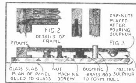
The method of casting a sulphur panel is illustrated above. The nuts, screws, bushings and other metal parts are first arranged in the mould according to a predetermined lay-out. The sulphur when hardened firmly retains these parts.
