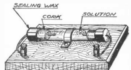
A small glass tube containing salammoniac solution and provided with terminals at its ends constitutes an effective polarity tester. When connected to a line the side at which bubbles are formed in the negative.
