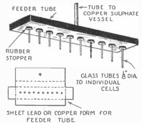
The feeder tubes can be very readily constructed of sheet lead or copper. The drawing above illustrates the method of construction.
