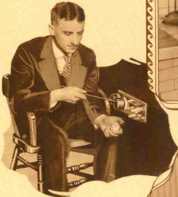
The Snow Fear Detector, an appliance for testing an automobilist's reaction to impending accidents.
