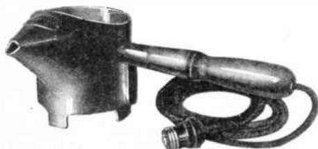
A very efficient electrically heated pouring ladle for applying the sealing compound for storage batteries. The heating coil is wound near the lip of the ladle so as to concentrate the heat there. To protect the hand a hollow wooden handle is provided.
