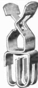
The Standard FAHNESTOCK Spring Clip, lead plated to prevent corrosion. Press thumb pieces together, insert wire, slip either over the poles or on the links of the battery for varying "B" voltage.
