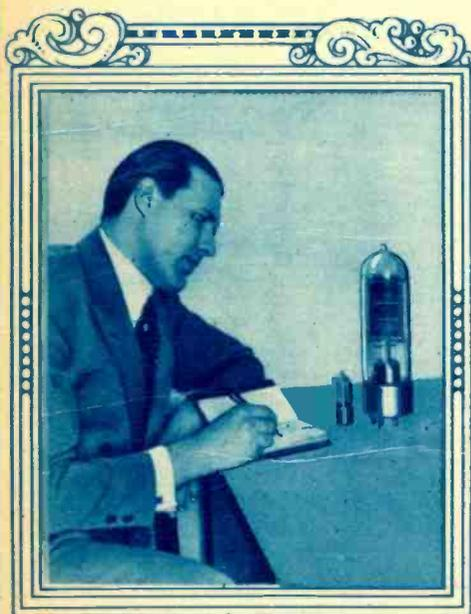
Chief engineer Willets is trying to calculate how long it will be before he will be able to discard the huge 250-watt transmitting tube and use in its stead the tiny five-watt tube shown alongside.
