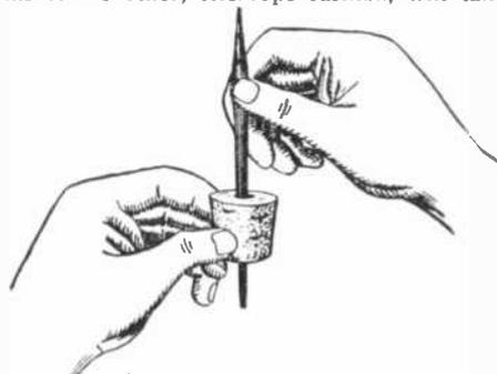
Making a hole in a cork, using a round file, commonly called a rat-tail file. This operation has to be done very nicely in order to get a perfectly cylindrical aperture.
