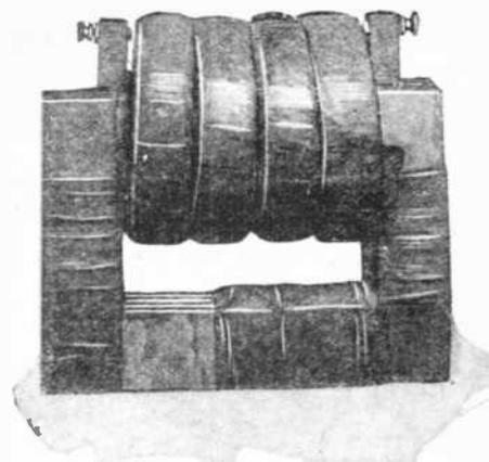
Fig. 3. An excellent type of home-made filter choke coil consisting of four large honey-comb coils and a silicon steel core.
