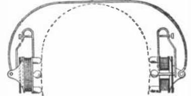
This is a head-set with very flexible diaphragms. Projections on the diaphragms press lightly against the temples. When a message comes over the telephone the pressure is varied, so that by the variations in pressure and by the duration of the periods of pressure, code can be received. Patent No. 1,531,543 issued to James J. Cooper, Atlanta, Ga.
