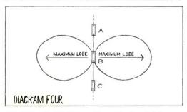
The dipole antenna pattern. The maximum gain lobe is at a right angle to the antenna, in both directions. Antenna gain off "the ends" of the dipole is at a minimum.
