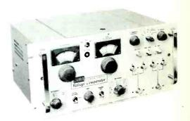
Model VC-12 (illustrated) features an accurately calibrated, variable two-mc rf signal which provides an rf reference voltage output variable from 1 millivolt to 12 volts.
