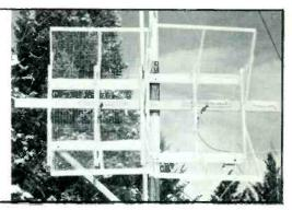
upper and lower stacks to cover two directions, or "broaden out" the main lobe beyond the limits of a single yagi. While this may partially solve the problems of coverage it can introduce severe ghosting, which the home receiving antenna is not able to cope with.
