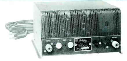
head-ends. In figure 3, the MLA-b is shown being used as a line extender. Up to 1700 feet of RG-11/U foam cable can be used between amplifiers (at channel 13). An MAC should be used every 3rd amplifier, to compensate for temperature changes, aging components, etc.
