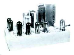
channel 2, 34 db max, gain channel 13. Mounts in pole box. 10,000 hour long-life tubes, all band amplifier, used as trunkline midsection compensator. Industry use. User net price: \$299.50.
