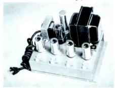
Unit gain, 5 db minimum. May be mounted at any indoor location. Matched inputs, separate slope adjustment for each output. Each output isolated from others and mainline. Four outputs. **User net price:** \$79.50.
