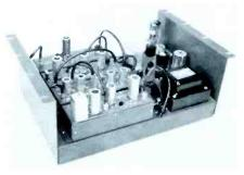
Unit must be ordered for specific channel. Operates from 115 vac, 60 cycles. 19 inch rack mounting. Output level, 60 dbm. User net price: \$562.20 (channels 2-6); \$752.-60 (channels 7-13).
