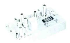
range 4-47 and 174-216 mcs. 15 db gain. Locates at bridging amplifier location in distribution systems. Converts signals in the 4-47 mcs. region to VHF channels 7-13 and then amplifies the converted signal to an appropriate distribution level. Plug in pads for cable equalization. **User net price:** \$115.50.
