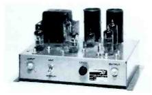
ing 2-6922/6DJ8 type. 35 db gain. Automatic overload control, adjustable slope, cascadable. Indoor or outdoor housings. **User net price:** \$170.00.
