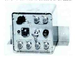
Weatherproof enclosure, 20 db gain control range, can be cable powered. Bridging amplifier-four outputs. **User net price: \$225.**
