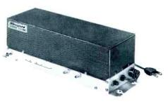
Unit has seven tubes, including two 6DJ8 type in cascode input stage. High and low band gain, 45 db. For use in driving up to 150 TV-FM receivers. Low band output, 1 volt. High band output, 1 volt. User net price: \$154.95.
