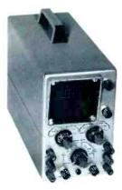
in four ranges. External capacity binding posts for lower sweep rates. Small, compact size measures only  $7\frac{5}{8}$  inches by  $4\frac{5}{8}$  inches by 11 inches. User net price: Kit, \$79.95.
