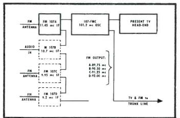
The CAS CATV/HEAD-end system is a method of providing several FM signals from standard FM or any audio source, with one basic system.
