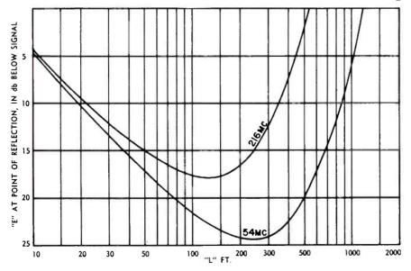
Figure 1. Minimum permissible return loss in RG 11/U coexial cable as a function of the distance between point of observation and source of echo.
