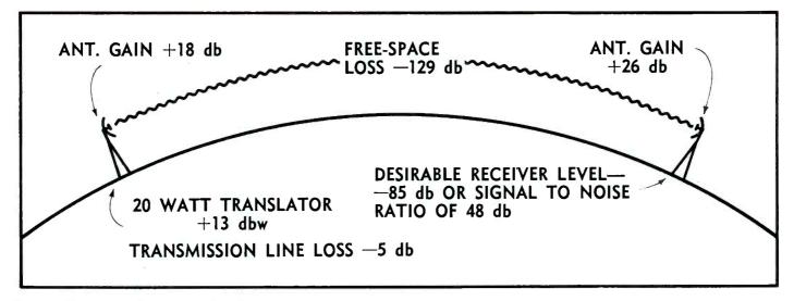
about 450 microvolts across 50 ohms or 1100 microvolts across 300 ohms. This is in agreement with practical experience with preamplifiers of this type. Desirable preamplifier signal is thus set at ---85 dbw.
