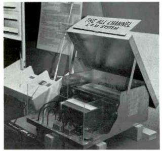
Telesystem Services Corporation of Glenside, Pa., displayed this chain distributed type all-channel trunk amplifier with separate external bridging , , , feeding cascade type distributor amplifier.
