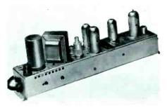
AGC controlled amplifier, Model MCSc. For single channel useage except for MCSc-FM which covers the entire FM band. Gain at least 46 db (low band); 38 db (ch. 7-10); 35 db (ch. 11-13). Maximum output; 1.0 volts for less than 1% cross-modulation; 2.0 volts for less than 3%
