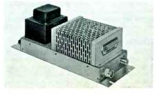
All-band line extension amplifier, Model 2098. Frequency range: 20 to 216 Mc. Gain: 27 db at 216 Mc. Cabinet mounting. Noise figure under 14 db over entire band. 10 db manual gain control. Low cost distribution amplifier with mainline dependability. 115 vac powered. Net: \$127.00
