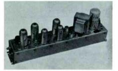
TV sound originator, Audio Master. Originates TV signal for any specified VHF channel. Provides crystal-controlled unmodulated video carrier plus sound carrier which may be modulated by any audio source. Audio carrier is 4.5 Mc above video frequency (TV Standards). Output impedance is 75 ohms. Net: \$175.00.
