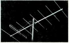
Single-channel, high band yagi, Model 718-HD. High band, cut-to-channel yagi designed for offthe-air pickup in extreme fringe areas. 8 element antenna with a forward gain of 13 db.
