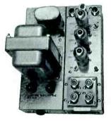
Low band bridging amplifier, Model BA-254. Four distribution line outputs. Gain: 20 db (bridging gain to each output). Maximum output level—5 channel operation: +42 dbmv (noncascaded). Manual gain control and plug-in attenuators provide ample control of gain. Self-
