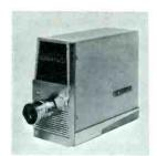
Automatic transistorized camera, Model TTVC-1-1. Self-contained, rugged, portable (15 lbs.), this camera transmits high definition (650 line resolution, 2 to 1 interlace) pictures. Has built-in automatic light compensator that adjusts for continuously changing light over a 2000 to 1 range. Video output, 1.25 volts. Usable picture may be obtained with as little as 1/2 foot candle of scene illumination with the standard F/1.9 lens supplied. Net: \$1950.00.
