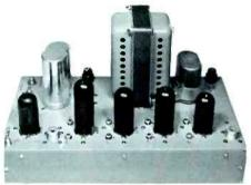
Low band trunkline amplifier, Model LRA-40C. Operates as low band VHF repeater. Incorporates ALC circuit. Gain at Channel 6: 40 db. Tilh: 7 db (Channel 6 over Channel 2). Noise figure: 7.5 db. Maximum output level: +50 dbmv (single amplifier--Channel 6). Uses 10,000 hour tubes and regulating transformer. "Sister" amplifier to Entron's HRA-400 for expansion to allband operation. Net: \$299.25.
