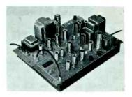
Push-pull sub-channel amplifier, Model SDX-440. Covers 4 to 47 Mc. 60 db second order beat suppression. Voltage stabilized transformer. Built-in AGC. Manual gain and tilt control. Builtin filter by-pass. Gain: 25 db (at 47 Mc). 6 db gain control range. Output: 36 dbj (operating). 75 ohm input and output impedance. F-61 fittings. Self-contained power supply. PNS.
