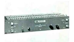
Low band amplifier, Model 211C. Covers 10-100 Mc. Gain: 33 db at 88 Mc. Choice of gain control, either manual or automatic using external 830 ALC or thermatic using external 832A Thermatic Gain control. Regulated, self-contained power supply. Cup core type transformers at the input and output provide excellent impedance match to the line. Rack or cabinet mounting. Net: \$328.00
