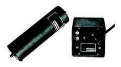
Single-channel preamplifier, Model AP-3. Designed for cable powering or can be battery powered. Power supply can be located up to 600 feet from pre-amp. Low noise figure on both high and low band. Gain: 40 db (low band) and 35 db (high band). 75 ohm input and output impedance. For storage battery operation, unit requires 9 vdc at 18 ma. Net: \$70.00.
