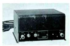
Line amplifier, Model MLA-C. Provides at least 40 db gain on all VHF channels. Separate gain controls for channels 7-13 and 2-6. Separate tilt controls. Maximum output (across 75 ohms) 2.0 volts per band for less than 1% cross- modulation. 3.5 volts per band for less than 3% cross-modulation. Net: \$93.50.
