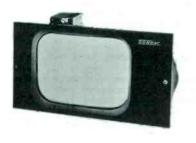
General purpose video monitor, Model CLB. Designed for continuous duty operation. Video response flat to 10 Mc for maximum resolution of 800 lines. Horizontal and vertical linearity within 2% of picture heighth. Taps available on horizontal output transformer so unit can be operated full scan or reduced scan. Built-in switch allows selection of either composite video or separate video and composite sync. Parallel jacks for loop-thru- operation. Net: \$315.00.
