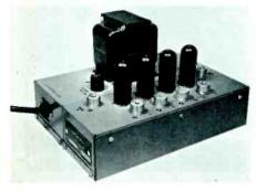
Low band bridging amplifier, Model BA-4C. Four distribution line outputs. Factory aligned to provide higher gain on low channels to compensate for normal tilt in the preceding trunkline amplifier. Gain: 3 db at Channel 2 and unity gain at Channel & ... channel bandwidth. 75 ohm thru line and 75 ohm distribution line output. RF isolation between input and output is 45 db. Net: \$112.50.
