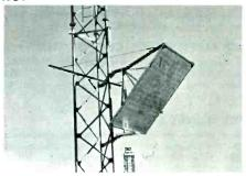
Microwave passive reflectors. Made of Reynolds aluminum interlocking extrusions. Three standard sizes;  $6 \times 8'$ ,  $8 \times 12'$  and  $10 \times 15'$ . Weight of reflectors is 140, 280 and 438 pounds respectively. Easy field asembly.
