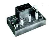
Line-bridging distribution amplifer, Model UBC-26B. Covers low band plus FM. Gain: 30 db minimum. Flat response. Maximum output: 47 dbj\* for 5-channel operation. Less than 0.3 of 1% distortion, single unit. Noise figure: 9 db or less. 3 db manual gain control range and plug-in pads (either P.I.P. or B.T.C. series). 75 ohm input and output impedance. Self-contained power supply. Can be used for line-bridging or cascading. PNS.
