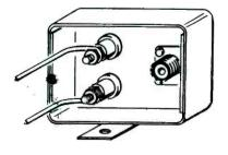
**Balun transformer, Model TB02-A.** 75 ohm to 300 ohm. Bandwidth: 2 to 300 Mc. Open wire line to cable. Weatherproof box. SO-239 connectors. Net: \$7.95.
