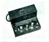
Low band line amplifier, Model LBB-MAN-50. 4 to 9 db variable tilt. Manual gain. Output: 45 db. Gain: 50 db at Channel 6. Utilizes electronic regulation. 75 ohm input and output. Self-contained power supply. Net: \$150.00
