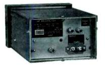
**UHF preamplifier, UAP series.** Six models to cover entire UHF range. Model UAP-7276 especially designed for MPATI areas and has 75 ohm input plus two 75 ohm outputs. Other models have 300 ohm input and output. Gain: 16 db at each of 2 outputs on UAP-7276 and 15 db on other models. Units have remote power supply. RF head is enclosed in rugged, irridited housing. Stabi-Life circuit for long tube life. PNS.
