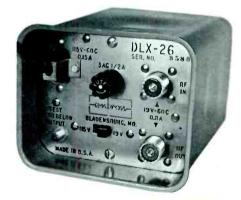
Low band line extender, Model DLX-26. Will extend distribution lines up to 2,000' using low loss cable or 1,000' using standard cable such as RG-11/U. Gain: 20 db. Noise Figure: 9 db. Self-contained power supply with power requirement of either 115 vac, 12 watts or 19 vac, 12 watts. (For remote powering use RPS-B power supply.) Output level:  $\pm 41$  dbmv. Net: \$120.00.
