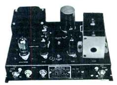
All-band distribution amplifier, Model TSC-4200. Gain: 30 db (minimum) low band, 37 db (minimum) high band. Maximum output: 1.7 volts low band (Channels 2-6 for 1% cross modulation), 1.7 volts high band (Channels 7-13 for 1% cross modulation). Tilt control range: 6 db low band, 4 db high band. Covers FM band. Separate high and low band gain controls. Ruggedized tube types. Net: \$71.00.
