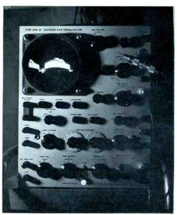
Oscilloscope presentation of video waveform showing color burst on most negative going portion of display.
