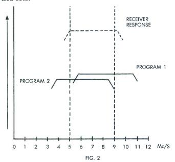
This arrangement of programme distribution, called the tete beche arrangement, relieves the problems of crossview between adjacent twin conductor circuits — see text.
