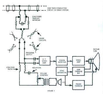
Block diagram of a multiwire receiver (basic Rediffusion), showing subscriber take-off network and audio feed to the loudspeaker.
