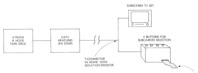
FIGURE 1. EDUCATIONAL UNIT IS FULLY COMPATIBLE, SIMPLE TO INSTALL.
