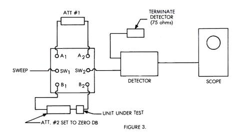
6. ATT #1 is provided to compensate for the residual insertion loss of ATT #2; the two units should therefore be of the same type.
