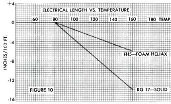
Fig. 10 Phase-temperature characteristics of RG-17/U and 7/8" foam Heliax.
