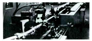
Fig. 1 Machine applying welded outer conductor over foamed cable core,
