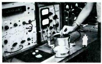
Fig. 2 Laboratory setup for measuring loss in dielectric.
