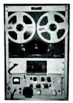
A complete music channel headend unit, the Davco Model MC-1100 Music Channel, has been announced by Davco Electronics Corporation. The unit is rack mounted and ready to plug in to any community antenna system. No other equipment is needed. It is completely wired and includes Tape-Athon tape deck with 10" reel capacity, pre-amplifier and Entron FMT FM transmitter, all as a complete integrated unit. Overall dimensions are 21" x 32".
