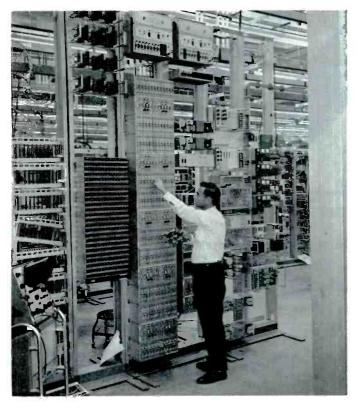
A microwave system receiving final check-out in the factory in Dallas.
