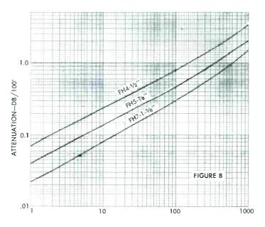
Fig. 8 Attenuation curves, 1/2", 7/8" and 15%" foam Heliax.
