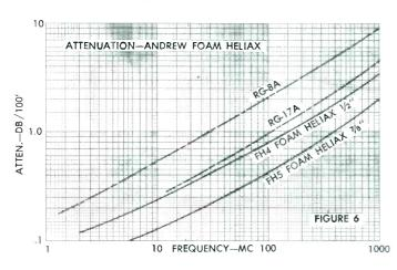
Fig. 6 Comparative attenuation curves for  $\frac{1}{2}$ " and  $\frac{7}{8}$ " foam Heliax.
