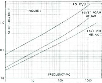
Fig. 7 Attenuation curves, 15/8" foam and air dielectric Heliax.
