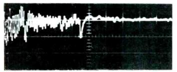
Fig. 5 Pulse measurement, RG8 on left, 1/2" foam Heliax on right.
