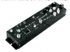
Transistorized all-band trunkline amplifier and bridger combination, Model ATMB-60. One 40-220 mc input, one trunkline and 4 bridger outputs. Average gain: trunk 30 db, bridger 7 db. Maximum output: trunk 50 db, bridger 45 db. Noise figure, 10 db measured at 220 mc. 10 db tilt control. Mainline gain control and tilt control; bridger gain control and tilt control. Cable powered AC/DC; regulated power supply. 75 ohm. Can cascade 40 units. Pole or strand box mount. Price: \$375.00.
