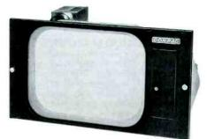
Rack mount 14" monitor, Model CLD14. Featuring both high and low voltage regulation, the CLD14 provides stability as AC line voltage varies from 105 to 130 volts. Designed for continuous duty, video response is flat to 10 mc assuring center resolution of 800 lines.
