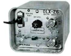
Low band line extender amplifier, Model DLX-26. Extends lines up to 2000 additional feet, using low-loss cable, or 1000 feet with standard cable. Average gain, 20 db. Maximum output, 41 dbmv. Noise figure, 8 db. Self-contained power supply; local or remote powered. 10,000 hour input tube. Mounts built-in or with mounting bracket Model QAB. Price: \$80.00.
