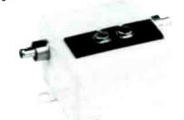
OF-320-FM subscriber connection device. Surface mounting. Ivory finish. FM tapoff attenuated 20 db. Push-on thru line fittings. 75 ohm input (thru line) and 300 ohm output (FM).
