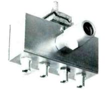
Directional coupler, Model DT-4. Four taps. For providing matched, isolated taps with directivity in distribution lines, 50 - 220 mc, 75 ohm, More than 30 db isolation. 0.7 db insertion loss. Loss per output 17 plus or minus 1 db. VSWR less than 1.1. Available with most connectors used in CATV. PNS.
