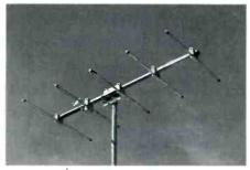
Ruggedized Proline. Machined all-aluminum ruggedized construction for MATV and CATV applications. Elements are 1/2", booms 11/4" round, heavy wall seamless hard-drawn aluminum tubing. No holes in booms or elements. Direct 52 or 72 ohm coaxial feed, available with all type con-
