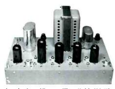
Low band trunkline amplifier, Model LRA-40D. Utilizes 10,000 hour input tube and 10,000 hour DC amplifier tube. Gain control range, continuously variable 0 db to full gain of amplifier. Average gain, 35 db. Output, plus 52 dbmv. Mounts any position on pole crossarm. Price: \$170.00.
