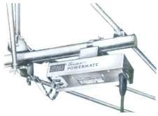
In announcing the new unit, Walter Goodman, Manager of Jerrold's Distributor Sales Division, said that the SPC-103 preampliifer has coaxial output achieved by a built-in matching transformer. It is contained in a metal weatherproof housing and is usually mounted on the boom of the antenna or on the mast, although it may be mounted on any flat surface.
