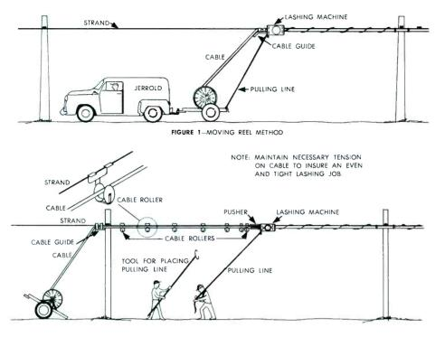
FIGURE 2-STATIONARY REEL METHOD
