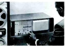
Available for 115v or 230v, 50-60 cycle single phase. Out put is 600 ohms, 0 dbm. Will feed up to 10 multi-channel recorders. All circuitry is solid state. Life
