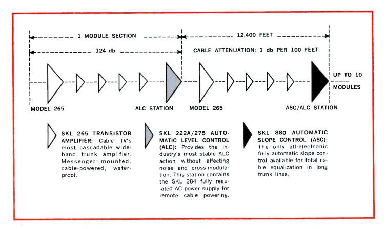
Each module section comprises five Model 265 Transistor Trunk Amplifiers cascaded in alternate sections with an ALC or ASC/ALC station. The module section length totals 124 db of cable. SKL's exclusive TEMPERATOR provides both thermal gain control and cable equalization at every Model 265 Amplifier. The
