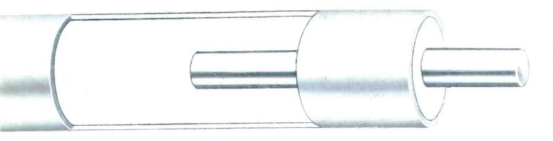
Now, the availability of 75 ohm Foamflex coaxial cable in four diameters - .412", 1/2", 3/4" and 1 5/8" - fills the needs of all-band CATV systems for rugged, high-performance cable in all required sizes. Foamflex, the original foam polyethylene dielectric cable, offers unequalled low loss for superior operation in community antenna and closed circuit television. Foamflex has a proven record in demanding applications in telemetry, missile guidance and microwave in addition to CATV.
