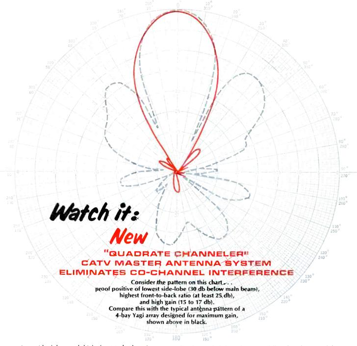
Low side lobes and high front-to-back ratio means rejection of all signals arriving at the antenna except those in the direction of the main lobe. The measured and guaranteed values on the antenna pattern above signify just one thing—elimination of co-channel interference.
