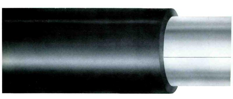
Sealmetic's positive moisture barrier makes the big difference. The Sealmetic sheath is hermetically sealed at the shield overlap, and is bonded between the entire outer conductor and the polyethylene jacket to form a unitized sheath. Moisture or humidity can't get between the shield and the jacket nor enter the core. The core stays dry and maintains the electrical characteristics of the cable.
