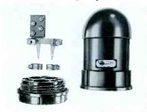
These terminals are the first to be specifically designed for direct burial under ground, or installation in a manhole or vault, according to the manufacturer. Since unit is hermetically sealed, the entire housing maintains pressure, hence terminations do not need to be potted in epoxy, or dammed off and by-passed.
