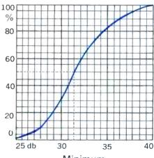
Minimum STRUCTURAL RETURN LOSS Distribution Curve
