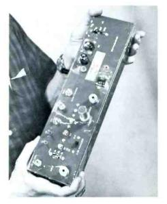
The amplifier was returned to Ameco Inc., the manufacturer in Phoenix for a complete check-out. In spite of the fact that it had been covered with silt and slime, the repair department reported that all it needed was a new rectifier diode to make it work like new.
