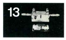
"Super Match" connectors permit full one inch engagement of cable conductor into spring finger contact area of connector body allowing for maximum thermal contraction of the conductor during extreme temperature variances—No more conductor "pull-out" problems.
