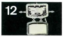
All input and output connectors are of the revolutionary new Viking "Super Match" true 75 ohm series.
