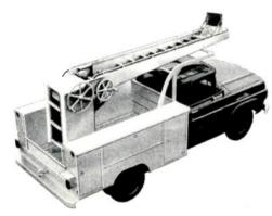
New HALLINE EM Series can be raised, extended and rotated to desired working position in seconds. Hydraulic elevation is controlled electrically by push button Topside elevation control optional. Extension and rotation are manually controlled. Available with extended platform heights from 26' to 30'. Designed for trucks with dual rear wheels.
