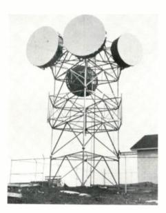
350 square feet of antenna surface, or the equivalent of six, 10 foot antennas per bay. Structural design is based on RS-222. All material is hot-dip galvanized after fabrication. Erection and detail drawings, foundation layout and anchor bolts are furnished with each Hex Tower. For further information contact Microflect Co., Inc., 3575 25th St. Southeast, Salem, Oregon 97302.
