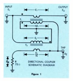
The ratio of these signals to the input signal (E) then provides the "tap value". in db, and insertion loss in db. This is shown in tabular form for various transformer turns ratio figures (N). Of course, these are ideal circuit values which neglect the Q of the coils and transformer losses. The values in the table are then the best possible theoretical values — and practical devices must be somewhat less in efficiency.
