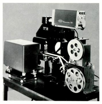
Heart of Trans-Lux Stock Quotation Program Service is this device which can provide two other sources of information (additional stock exchanges, local news or other announcements) along with the New York Stock Exchange tape.
