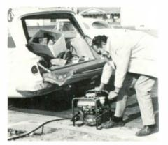
1,500 watt portable generator weighs only 40 lbs. and provides plenty of power for field use of electric heat guns.
