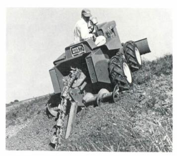
60-horsepower trencher is applicable for distribution line or main trunk installations, and is convertible to vibratory plow. Trencher provides trenches of up to 24 inches in width, and up to 7 feet in depth.
