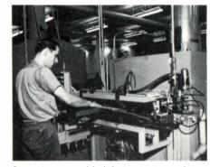
Loosely assembled helical-wire subsetpass under a cascade of liquid adhesive, then enter the drying oven where they are bonded into permanent assemblies.
