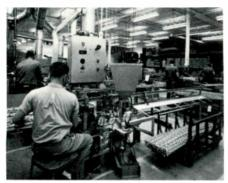
As finished "sets" pass through this machine, inside surfaces of the units are sprayed with a quick-drying adhesive, then coated with a special grit to increase the holding power of the hardware.
