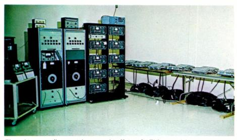
The "white screen" tester (above) used in Kaiser CATV's tests delivers signals very similar to broadcast television signals.
