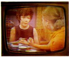
The color pictures above were received at the end of the 42-amplifier cascade in the Merced-Atwater mid-band tests.
