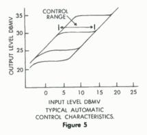
from their use. Figure 5 shows a typical set of control characteristics.
