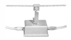
at Ch. 13. Flatness  $\pm 1/4$  db. No visible cross modulation (12 channel loading) at  $\pm 46$  dbmv (Ch. 13P). Noise figure 11 db. Variable duty cycle pulse type switching power supply for maximum efficiency and minimum current drain. Does not require AGC control. Silicon transistors throughout. For in-line mounting.
