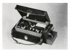
and portable. Frequency range: 54 to 108 mc; 174 to 220 mc. Four sensitivity ranges: 10 microvolts to 1 volt; 33 to +60 db. Accuracy: ±1.75 db. Input impedance: 75 ohms. Connectors: Type F. Batteries: 2 standard 9 volt. Price
