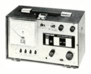
ments) in two ranges: VHF (52-216 mc) and UHF (470-890 mc). Sensitivity variable from 100 uv to 3 v full scale meter deflection. Reads both average and peak level. Fully solid-state circuitry. Battery or power line operation. Fully regulated power supply, no adjustments necessary. \$395.00.
