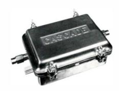
1/20 has a maximum gain figure of 22 db, and a recommended spacing or operational gain of 20 db. This recommended oprational gain includes up to 10 db of flat loss. Gain control range is tilt compensated, 8 db continuous. Both the RF circuit and the power supply circuit are of the Cascade printed circuit module design, which permits instant insertion or removal. The housing is a cast aluminum weather-and water-proof. Price \$119.50.
