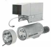
TCA-1 Local Control Adapter. Adapts the G.E. TE-22 remote back camera to local control, eliminating the need to transport a separate camera control unit for "on location" pick-up, and expanding single-camera economy to serve dual functions. Equipped with a video output connector for attachment of a viewfinder, mechanical focus control, and electrical controls including target, focus, and beam. Five and one-half inches in diameter, 2¾" long.
