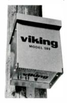
voltage from 95 to 130 VAC, and within 2% for load variations between 2 and 6 amperes. Unit has built-in automatic re-set circuit breaker; an RF/power filter provides minimum of 60 db isolation between power lines and RF terminals. Unit may be rack, wall or cabinet mounted, and has meter for constant monitoring of output current.
