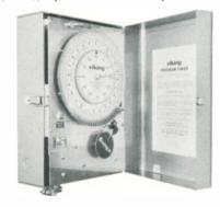
curately controlled by a set of cams operating micro switches. Unit is synchronous motor driven for split second accuracy. All adjustments are made on front of timer. Can remotely control wire system.
