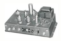
trol to -20 db. Tilt controls, low-band 6 db, high-band 5 db. Maximum output is 64 dbmv per band for less than 1% cross modulation. Power requirements, 45 watts, 117 VAC.
