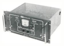
A.G.C. and carrier level controls. Has automatic substitution carrier (switched by solid state devices) with variable sensitivity and sub. carrier level control. Crystal controlled input and output mixer/oscillators together with separate
