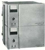
vides a complete transmitter or receiver in 10½ inches of rack space. High transmitter output (minimum of 1 watt), and frequency stability (plus or minus .005%) for reliable performance. Differential Phase of ±0.25 degrees, and Differential Gain of ±0.25 db. Available in models for 6-8 GHz common carrier and 12-13 GHz C.A.R.S. bands.
