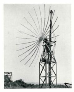
**30 Ft. Parabolic Antenna.** All channels from a given area can be received with one antenna and one feed. By positioning feed in parabola, a null can be placed in direction of undesired channel. Covers all UHF and VHF channels; steel and aluminum construction.
