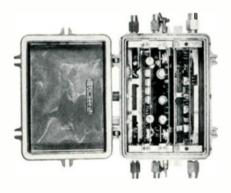
amplifier in combination with the bridging distribution amplifier circuit, and achieves a maximum gain of 30 db, with a recommended operating gain of 27 db. Maximum noise figures are 19 db low band and 21 db high band, and are corrected for the directional coupler within the amplifier. The true amplifier noise figures are 9 db low band and 11 db high band. Price \$395.00.
