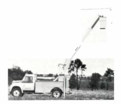
cat digger-derrick. The insulated jib and crossarm can be used as a jib parallel to the ground for approximately 5 ft. of extra horizontal reach or it can be hydraulically tilted to in-line with boom for approximately 7 ft. of extra vertical reach. The unit can be stored on top of boom when not in use, and has a 500 lb. capacity.
