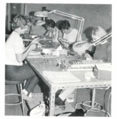
After all components have been attached to the circuit boards, they receive a preliminary inspection for physical construction (shown above) then go through electronic tests, before reaching the next stage of amplifier assembly.
