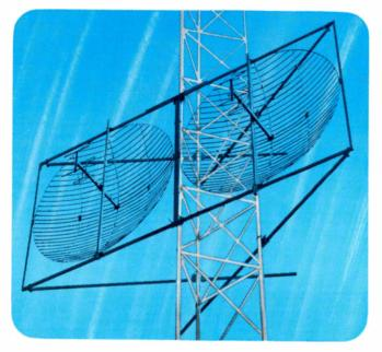
**Parabeam Broad-band UHF Antennas** consist of modular packages of small grid-type dishes that offer only 1/10th the wind load of solid surface dishes claiming equivalent gain. What's more the grid-type construction does not require the large structural back-up members that contribute to wind load.
