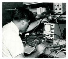
Joe Zarowny, who heads test and alignment operations, is shown aligning a lowband line extender.
