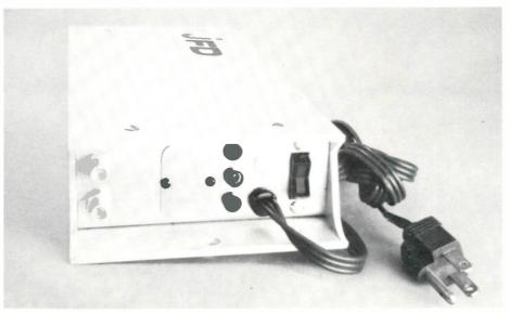
Figure 2: Typical solid state MATV head-end amplifier. This unit is capable of overcoming up to 52 channel distribution system loss.
