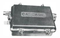
temperature level control. Manufacturer's specifications list maximum output capability as +48 dBmv; maximum gain as 25 dB; operational gain as 22 dB; frequency range as 50-220 MHz; Input return loss as 16 dB; output return loss as 12 dB and noise figure as 10 dB. The price of the unit is \$149.50.
