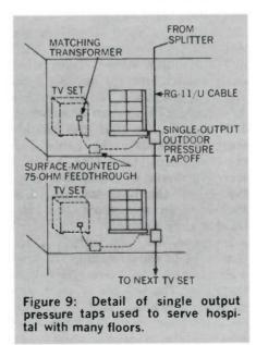
Suppose, however, that the building is taller than 4 stories. In this case, you'll need vertical trunklines as shown in Figure 9. Rather than
