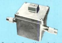
Compact unit provides moderate gain (or loss) at feeder tapoff, and supplies amplified signal to four outputs. Gain may be adjusted over a 13db range, from-8 to  $\pm$ 5db with respect to input. Maximum input is  $\pm$ 20dbmv at 5db gain, and  $\pm$ 33dbmv at-8db gain, and through-line insertion loss is less than 1db. Return loss at input, output and taps is 16db. Frequency range is 50-220 MHz,  $\pm$ 5db, and output capability is  $\pm$ 25dbmv.
