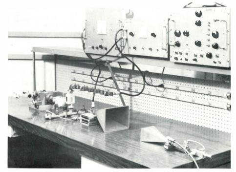
Figure 1: AML Breadboard Transmitter and Receiver.
