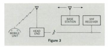
extend talk-back range, as illustrated in Figure 3. These subscribers could be even better served by providing individual narrow band strip amplifiers or heterodyne amplifiers at the head-end for their specific frequencies. Such subscribers would undoubtedly use fixed-tuned receivers.
