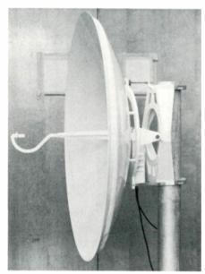
Figure 11: Prototype AML Receiving Antenna.
