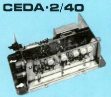
Self-powered four-stage distribution amplifier, equally suited to trunk/feeder application and MATV type distribution within hotel and apartment buildings. Offers 40db gain and +50dbmv output capability. Gain and tilt controls provide compensation for 30db of cable and 10db flat loss to 40db flat loss. Requires only 11.7 watts at 117 VAC. Ideal replacement for older tubetype equipment.
