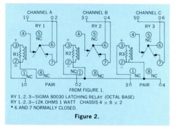
operated by the N.D.S. Figure 2 shows the schematic of the relay circuits which are built up on a  $4'' \ge 8'' \ge 2''$  aluminum chassis. Figure 3 is the circuit of the tiein to the TeleMation unit coaxial relay holding coils for the channels involved.
