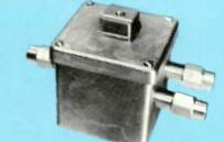
CELS is a passive line splitter, providing equal output to two trunk or feeder lines. Unique construction allows circuit board to be positioned to use any of the three connectors as input, and other two as outputs. Input and output return loss is 18db over 5-240 MHz range, and tap-to-tap isolation is 18db. Splitter loss is 3db at Ch. 2, and 3.5db at Ch. 13.
