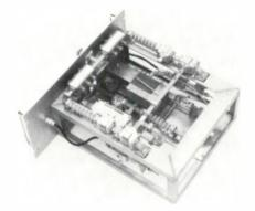
Figure 3: Experimental Transmitter Up-Converter.
