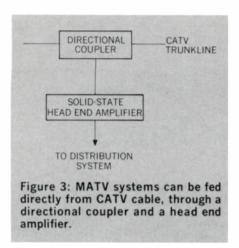
feed it only about 20 dB, you would need a head-end amplifier such as that shown in Figure 2. The complete head-end for this school system is shown in Figure 3.
