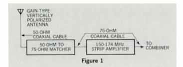
distribute Weather Bureau, land mobile and VHF marine (150-174 MHz) radio signals by installing a strip amplifier for this frequency range at the head-end, as shown in Figure 1.
