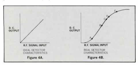
changes in output levels. Even in the regions of slight curvature small changes in RF input will produce accurately proportional small changes in DC output. Thus, if we calibrate our equipment at the carrier level we are to use during tests and at a sufficiently small modulation index, we can expect to obtain excellent accuracy even if the overall detector characteristic is not suitably linear over the whole range.
