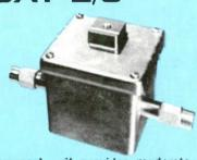
Compact unit provides moderate gain (or loss) at feeder tapoff, and supplies amplified signal to four outputs. Gain may be adjusted over a 13db range, from-8 to +5db with respect to input. Maximum input is +20dbmv at 5db gain, and +33dbmv at-8db gain, and through-line insertion loss is less than 1db. Return loss at input, output and taps is 16db. Frequency range is 50-220 MHz, ±.5db, and output capability is +25dbmv.
