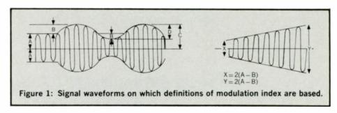
defined from this pattern as (Y-X)/(Y+X) which can be shown in the sine wave case to be equal to B/A or m c. However, if the modulating signal is not symmetrical as would be the case for an "off air" signal, (Y-X)/(Y+X) will not, in general, be equal to m c.
