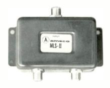
maximum insertion loss with typical insertion loss of 3.75 dB, and an input return loss of 16 dB. The device accepts F-59 connectors and is available for immediate delivery. Price of the MLS-II is \$2.50.
