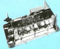
Self-powered four-stage distribution amplifier, equally suited to trunk/feeder application and MATV type distribution within hotel and apartment buildings. Offers 40db gain and +50dbmv output capability. Gain and tilt controls provide compensation for 30db of cable and 10db flat loss to 40db flat loss. Requires only 11.7 watts at 117 VAC. Ideal replacement for older tubetype equipment.
