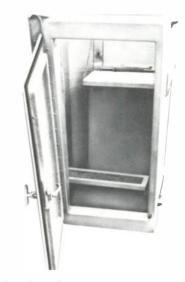
ing lengthy operations. The chair is hinged to the inside wall of the bucket and swings up out of the way when crewmen must work standing up. For further comfort, a footrest can be lowered from the bucket wall. A large 39 x 18 in. sidewall door provides easy access to the bucket and eliminates crawling over the bucket lip to enter or exit.
