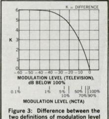
two definitions of modulation level vs. modulation level.
