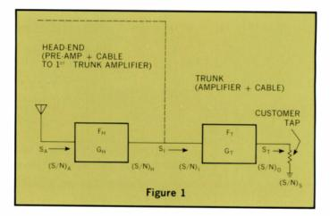
It is assumed, in accordance with practice, that the head-end AGC compensates for any antenna signal, maintaining the signals into the trunk amplifiers constant. Also, the S/N ratios shown in the above diagram are the individual S/N ratios, considering each section separately. Their combination, which gives the resulting S/N ratio for the overall system,  $(S/N)_S$ , will be illustrated by the following examples:
