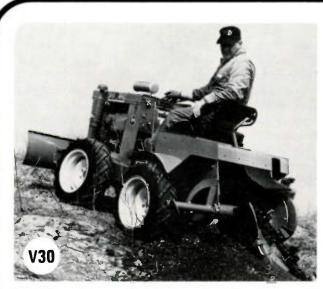
The 30 h.p. trencher that delivers everything you expect from utility and service line equipment, plus a full line of options including backhoe, Roto Witch boring unit, and offset pivot for tight work. You get 4-wheel drive, full hydraulic control, power steering, uphill ability and sidehill stability, and trenching up to 24 fpm.
