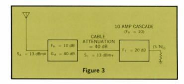
be 20.4 dB. This yielded an  $(S/N)_0 = 51.6$  dB. (First case). He then postulated a reduced antenna signal of 3 dBmv while maintaining the amplifier signal levels, or, in effect, a good head-end AGC. He recalculated the overall system noise figure to be 13.2 dB. This yielded an  $(S/N)_0 = 48.8$  (Second case).
