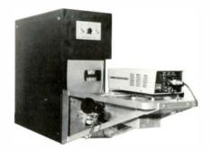
photographs or other data. It also has a built-in high precision time and temperature dial. It cycles every 2 minutes, is compact and comes with its own camera.
