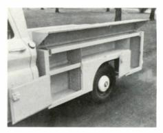
the hazards of a protruding door. Shelving or parts drawers remove easily for interchange. Optional items include: lift gate, material hooks and ladder racks. FSM's are available in four models, 72" to 101" long, to fit  $\frac{1}{2}$ ,  $\frac{3}{4}$  and one ton narrow box pickups.
