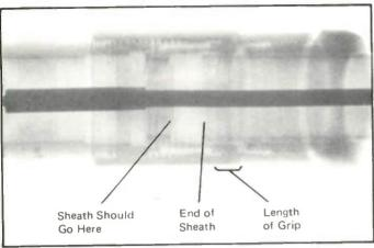
This splice shows questionable quality. Center conductors are into collets OK, but sheath does not go far enough into connector for proper grip by clamps inside. Center conductor was left too long before installation in splice.
