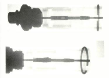
Top: cable test adapter connector which was intermittent. Note poor fit of center pin into collet. Bottom: the same connector after repair with solder.
