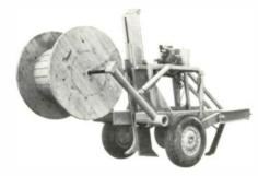
safety relief spring, plow tooth vertical adjustment from 0" to 50" and front jack stand. Plow tooth thickness from 2" to 4" is available and the unit buries material up to  $3\frac{1}{2}$ " O.D. or larger with modifications.
