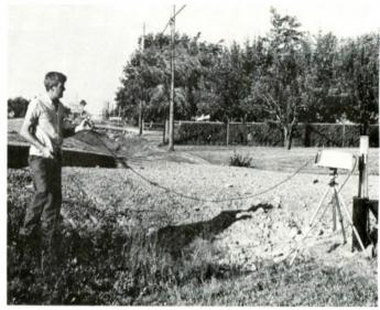
After preparing film and X-Ray unit, the technician steps well back and uses remote control cord to actuate X-Ray mechanism.
