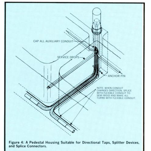
proofed for buried plant use, are presently available from two CATV equipment manufacturers. One firm'stapiscompletely potted with a polyurethane foam material and the case is anodized for corrosion protection. The other firm uses an epoxy resin over the entire electronic circuit board within the housing which affords complete moisture protection. Protection to all splitter devices is also provided by the use of the polyurethane foam potting method.
