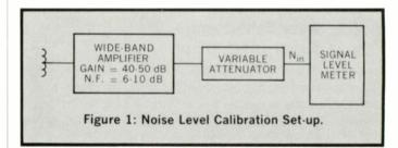
(5) With this connection the noise level at the input terminal of the signal level meter is the output noise level of the amplifier diminished by the attenuation of the attenuator:
