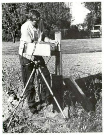
The portable field X-Ray unit can be mounted on a tripod and used to check splices made in pedestals. Here, the technician tapes polaroid film to the splice.
