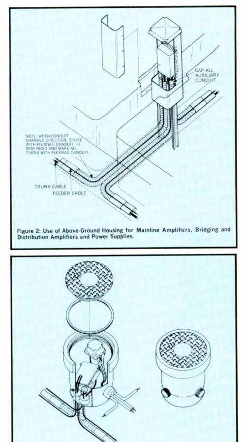
Figure 3: Use of Underground Housing Suitable for Placement of Line Extension Amplifiers, Directional Taps, and Splitters. to grip, liberal use of pulling compound and continuous steady pull with no stopping during any length of pull. If two or more cables are to be pulled into the same conduit, they should be pulled together and not separately.
