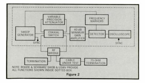
adaptors will produce frequency sensitive reflections sufficient to vitiate test results. (c) Jumper cables between the coaxial switch and RF bridge should be matched in type and length to jumpers between the coaxial switch and precision attenuator. This will minimize extraneous deviations between reference and test circuits. Otherwise, annoying (frequency
