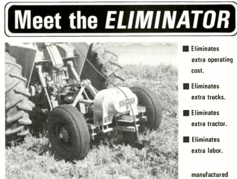
Introducing the new Lubbock plow The ELIMINATOR The benefits are cable or pipe laid at uniform depth. simple in design, yet rugged operated at optional 30% to 50% less drawbar peed 540 or 1000 RPM putI than required by static ripper. standard tractor with 3 point hitch handles the new Lubbock plow
