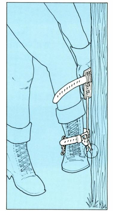
1. Select a location on the pole that is free and clear of gaff marks, cracks and knots.
