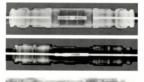
X-Ray of cable splice on "wet" film (no screen medical) showing detail of improper splice. Cable ends have just been jammed into splice with no center conductor at all.
