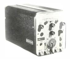
variations greater than 10,000 to 1 is provided. Other features of the camera include gamma correction and video polarity reversal and white peak clipper.
