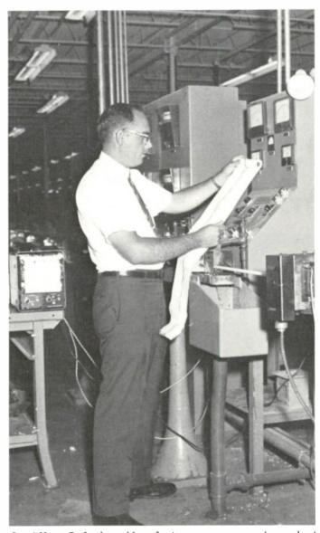
J. Allen Oxford, cable plant manager, examines chart recording of diameter and capacitance from continuous monitoring as core is extruded. Polyethylene foam is extruded around the pre-heated copper center conductor. From this point, core passes through series of cooling troughs to take-up equipment.
