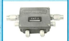
Line powered 50-220mHz tap has gain range from -8db to +5db with respect to input, and output capability of + 25dbmv (11 channels 100% synchronously modulated: Ch. 13 crossmod -57db). Return loss at input, output and taps is 16 db or better. Insertion loss at Odb gain (Ch. 13) is less than Idb with 3db tilt.
