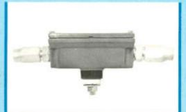
For insertion in trunk and feeder lines where an unequal split is needed, CEDC-1/8 and CEDC-1/12 provide tap values of 8 and 12db, ±1db. Through-line insertion loss is 1.5 and ldb, respectively. Input and output return loss is 18db over the 50-250 mHz bandwidth, and directivity is a minimum of 18db.
