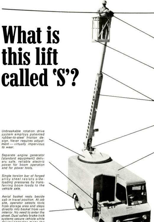
Three direction-oriented toggle switches control boom movements. Optional single omnidirectional control initiates boom travel in any direction or combination of directions in response to light hand pressure.
