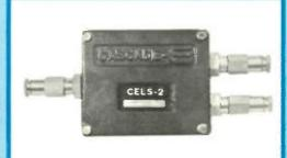
CELS is a new passive line splitter, providing equal output to two trunk or feeder lines. Input and output return loss is 18db over 50-250mHz range, and tap-to-tap isolation is 20db. Splitter loss rises from 3db at Ch. 2, to 3.5db at Ch. 13. Both strand and pedestal models are offered.
