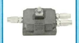
Convenient splice box connects cables and provide separate AC and RF test points. AC test point is marked in red as a reminder that FSM is not to be connected. RF test point is -30db, ± 1db. Return loss 25db, insertion loss .25db. Optionally, insertion loss may be reduced to .1db by removing RF test point components.
