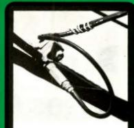
Line-guard No. 1 is inserted between pressure - tap and house drop connector to disconnect service.
