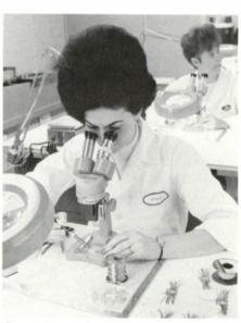
One step in the assembly of thin film microcircuit for Superband amplifier.
