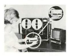
panel of the Videocorder. The new control unit is designed to permit users to select an isolated portion of the video tape for automatic, continuous viewing. The unit is adaptable to, and interchangeable with Sony's Models EVR-200 and EVR-210 remote control panels; it can also be installed on the EV-200R Videocorder. The EVR-210-A lists for \$295; the unit plus installation in standard Model EV-210 is \$625.
