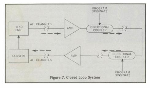
transmission is essentially in one direction, which is around a closed loop. Therefore, crosstalk, "singing," and echo are not inherent problems of this system.
