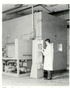
The firm's environmental chamber is used to evaluate amplifier performance.
