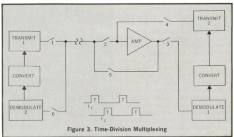
(b) Time-Division Multiplexing—This arrangement, which is essentially a sampled data modulation process, is shown in Figure 3. Although it is a theoretically possible system, its use at the high frequencies of the cable system is limited by present state-of-the-art techniques of time sampling. It is described here only as a hypothetical case of its application to bi-directional cable systems.
