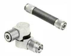
be twisted through 360°. When used together, these devices are engineered to permit movement in all three dimensions. Insertion loss of either of the new components is rated at less than 0.5 dB over a frequency range of dc to 12.4 GHz with SWR less than 1.1.
