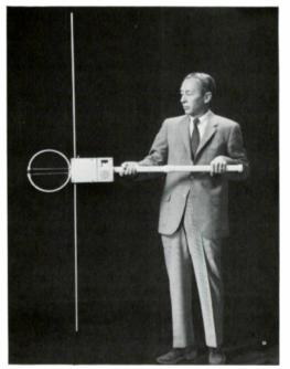
In operating the Noise Source Locator, the operator stands under the power line which is suspected to be the source of trouble, and determines very quickly the direction of the noise source with respect to his position. He then can walk in the direction of the source until it is found. As, for example, the noise is caused by minute arcs in the line hardware on a pole, the TNL2 indication will quickly decrease once the pole is passed. In this way little time is lost in finding
