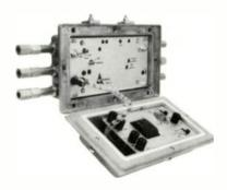
+32 dBmV output, measured according to NCTA standards. Other characteristics listed by the company include a noise figure of 10 dB and input and output return loss of 16 dB. The plugin modules are designed to fit a common waterproof housing, with built-in transformer-type power supply. Available modules include optional AGC operating from pilot carrier or from composite signal levels.
