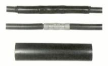
mastic coating and are available with both standard and heavy wall thicknesses. Upon applying heat, the sleeve is designed to shrink to conform tightly to the splice while the mastic melts and flows to provide a watertight seal.
