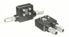
All connector ports have the Craftsman Sleeve to accept connector sealants such as heat shrinkable tubing or tape. The 2600 incorporates a corrosionproof poly carbonate outer case that encloses the die cast aluminum inner case which is internally potted with low density foam.
