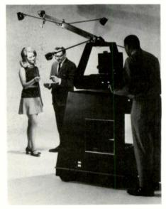
No equipment need be dismounted for movement or storage. The lights fold in, the boom retracts and the boom and camera mount tilt to the full-down position. In this position, the unit can easily be moved from room to room by one person. With all elements in the storage position, the TV Dolly-Lite will pass through any standard 32-inch doorway, so any room can become an "instant TV studio."  $\mathbf{w}$
