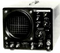
Patterns on the flat-face, hignsensitivity 5" screen are exceptionally bright. There's no "dot blooming" with the 1460; 1650 volts on the accelerating anode insure sharp patterns at fast writing speeds of up to 0.1 microsecond/cm (with x5 magnification). The only tube in the 1460 is the CRT, all else is solid-state. It is priced at \$389.95.
