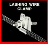
Permanent termination for lashing wire at the pole. Aluminum alloy plates fit and hold ¼" strand. Hot dipped galvanized washers and nut hold lashing wire.
