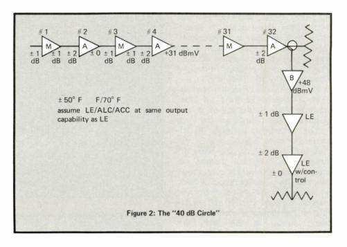
cross-mod. and with a reduction in levels, the *trunk* exposes noise. A second situation should be obvious from this design. That is, this system will require daily, weekly, monthly, or seasonal rebalance. The frequency will be determined by the system locale.
