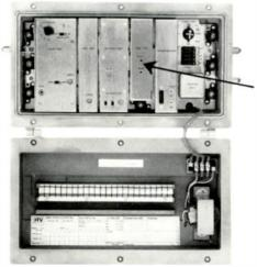
Sub VHF amplifier or Jumper Module. (Separation filters under base plate.)
