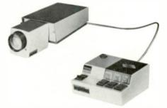
The remote-controlled unit allows operation of the zoom lens under certain circumstances where it is not possible or desirable to have an operator near the camera. The zoom control unit has a speed range of 4 to 40 seconds. A special clutch arrangement provides an immediate stop of focus, zoom and iris motors without slowing down.
