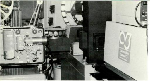
With a film chain incorporating two 16mm motion picture projectors, a double-tray 35mm slide projector and a Kodak multiplexer, Channel 3 can cablecast entire programs or intercut into studio taping sessions.
