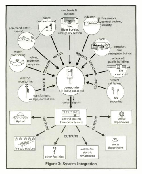
the transponders are received at the central station and fed to readout equipment, which indicates status of the monitored points.
