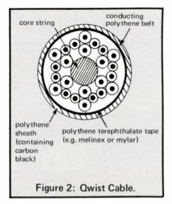
balanced 130 ohm transmission line, providing low transmission loss with minimum susceptibility to interference and cross-talk.
