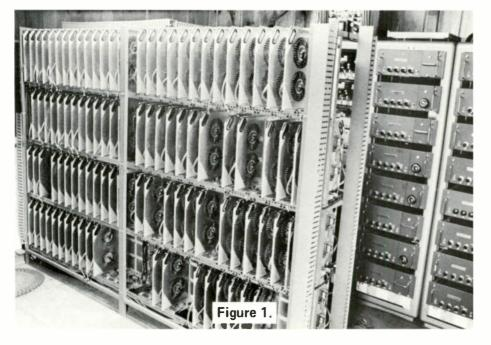
exchange operate at a 12 ohm impedance level, unbalanced. A system of hybrids and baluns drives balanced 130 ohm subscriber service lines at 700 millivolt level.
