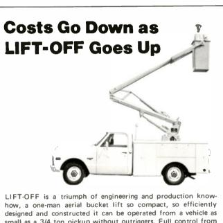
designed and constructed it can be operated from a vehicle as small as a 3/4 ton pickup without outriggers. Full control from the fiberglass bucket by recessed push buttons permits one man to be totally self-sufficient with maximum satety. Fully articulated, rotating booms allow complete freedom of movement. LIFT-OFF'S compact power plant provides a maximum of 2500 watts of power, sufficient for most electrical tools. Duplex outlets are located at the bucket yoke and boom base.
