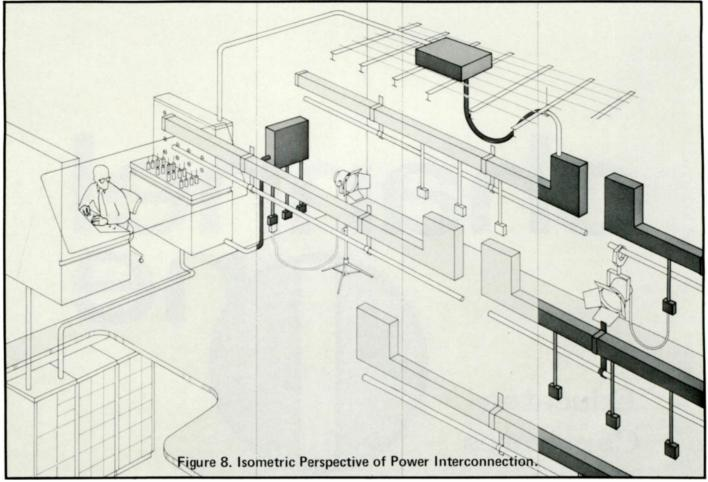
The first section above shows the three basic components of a dimmer system: control console, patch panel (behind the technician) and the dimmer rack (in basement). The second section emphasizes the wall outlet box. The third section emphasizes the grid iron junction box and the last section emphasizes the plugging strips.
