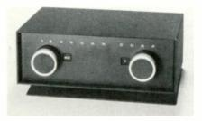
Packaged in a cabinet of modern design, these attenuators feature low VSWR and flat frequency response. Calibration data is supplied with these instruments to increase their usefulness. Calibrated attenuation data is supplied at 30 MHz, 500 MHz, 1000 MHz and 1500 MHz. These attenuators are useable to above 2000 MHz, with slight degradation in the performance specified at 1500 MHz.
