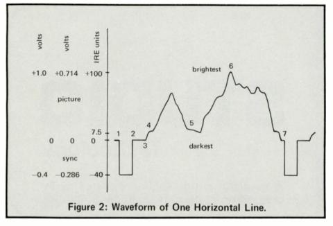
standardized, so that a signal which is positive with respect to zero contains picture information only. Negative signals are synchronizing pulses.
