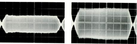
These two photos show oscilloscope readings of radio frequency (RF) output of standard tape (left) compared with almost double the output (right) of the new "High Energy" videotape.
