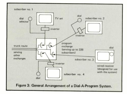
operating the dialing system, the inverter section is powered by a separate 115 VAC line cord. A conventional RG-59U coaxial cable connects the inverter to the subscriber receiver.
