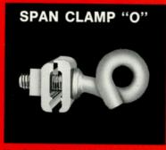
Used to take off house drop wires or cable along the span. Positive control installation. Round hook  $\frac{1}{2}$ " steel, Plates are aluminum alloy for  $\frac{1}{4}$ " strand.
