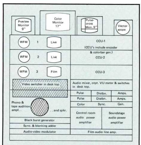
Figure 5: Desk-top twin racks without sloping turrents accommodate all necessary equipment with some monitors placed on top.
