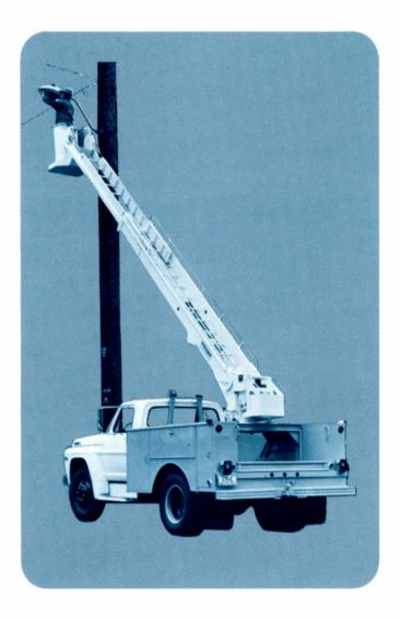
Quality and performance are foremost in the design and construction of the EME Bridge Mount Ladder. This is reflected in the strength and lightweight of the unit. The rigid lower section offers all welded steel reinforced construction. The lightweight upper section is fabricated from reinforced fiberglass which resists unfavorable weather conditions and offers maximum insulation.
