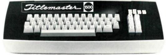
Every TV and CATV operator needs it . . . and even the smallest can afford it! Titlemaster is a low-cost, self-contained electronic character generator designed for broadcast, CATV or CCTV.
