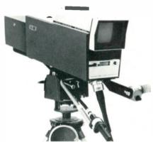
The IVC-500A offers significant new features compared to previous IVC cameras but incorporates a silicon diode tube in the red channel and Plumbicon tubes in the blue and green channels.
