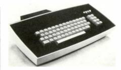
This capability makes it possible to display one page of the channel while composing, editing or previewing any one of the remaining three pages of the preview channel. The audio record/playback interface allows offline storage of additional display information. The generator meets EIA RS-170 video standards and RS-232 data standards for universal application.
