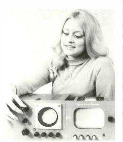
tion with a high-resolution 5" picture monitor. The assembly, WV-063, requires 7" of rack space and is designed primarily for placement of one such array on the output of each camera in a studio system, although it may be connected anywhere in the video circuit.
