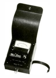
The unit also contains a 0 to 60 Volt AC and DC voltmeter. Line voltage can be measured, and amplifier and power supply trouble shooting can be performed with the same instrument.
