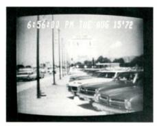
Timing accuracy is established either by power line frequency or use of an external standard. A 100-year calendar circuit automatically corrects for length-of-month and leap year variations. This assures continued
