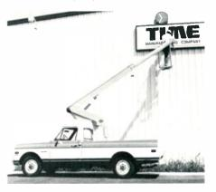
Use of an aluminum upper boom with a simplified drive and power system have resulted in a total unit weight of 1200 pounds.
