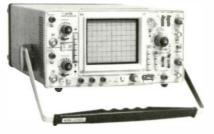
portable oscilloscopes, the 465 and 475. The 475 features 200 MHz at 2 mV/cm. The 465 has 100 MHz bandwidth at 5 mV/div. Both achieve full bandwidth at their highest sensitivity settings and contain a big, bright 8 cm by 10 cm display with risetime graticule. The 475's sweep speed is one nanosecond with X10 Mag.
