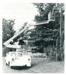
According to the manufacturer, the unit is designed to be mounted on a 3/4 ton chassis having a 56'' C.A.
