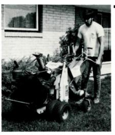
No other machine of its kind can equal PIPE PIPER for speed, maneuverability, and low labor cost. You can bury wire, cable, or flexible pipe around corners and obstacles in one continuous operation. There is no damage to the finest turf and no trench to fill. Constant burying depths of from 5 to 14 inches are easily maintained with one setting. PIPE PIPER is easily transported in a van or trailer.
