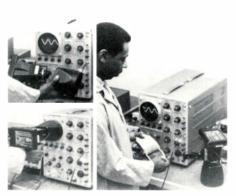
presently on the market. Unlike most permanently-mounted cameras, a single handheld CR-9 can easily be used with more than one oscilloscope at multiple installations. Because of its portability and light weight, the unit can easily be carried from one terminal to another. The CR-9 is designed to accept any of 8 interchangeable, light-tight hoods in
