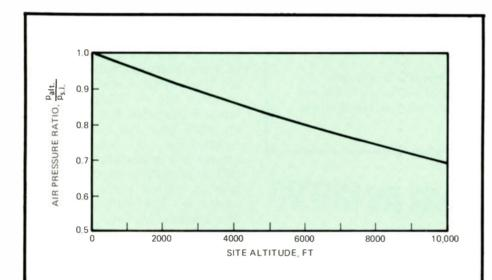
Figure 8: Air Pressure Ratio as a Function of Site Altitude (For Calculation of Altitude Correction Factors for Solar Radiation and Free Convection).
