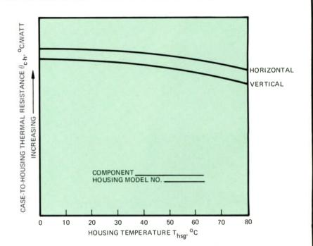
Figure 10. Typical Plot of Component Case-to-Housing Thermal Resistance as a Function of Housing Temperature and Housing Orientation.
