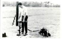
Basic power unit is 5 hp earth drill built to drill both horizontal and vertical. Drill can be used to feed trees, drill access holes, plant trees, as well as many other jobs.
