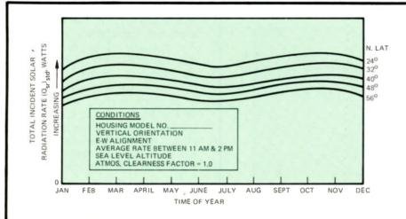
Figure 7. Three-hour Average Total Solar Radiation Heat Rate (Direct + Diffuse) Incident, at Sea Level, on a Vertically-Oriented, EW Aligned Housing of Specific Dimensions.
