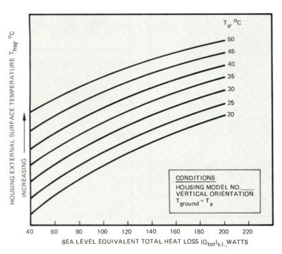
Figure 9. Housing External Surface (Reference) Temperature for Combined Free Convection and Radiation Heat Loss From a Housing of Specific Design as a Function of Sea Level Equivalent Total Heat Loss and Ambient Air Temperature.
