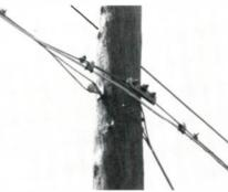
Easy-to-install FALSE DEAD END is wrapped on by hand without cutting the strand. Mechanical strength equals the strand on which it is applied. Slim profile improves appearance.
