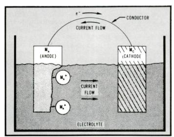
Figure 3A. Illustration of principle of galvanic (dissimilar metal) corrosion, showing the four key elements – anodic metal, cathodic metal electrical contact or conductor, and electrolyte – which must be present for galvanic corrosion to occur.
