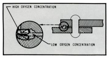
Figure 7. Sketch illustrating the occurence of the oxygen concentrations form of concentration cell corrosion.
