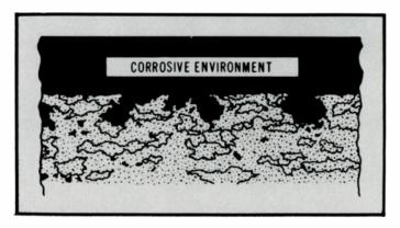
Figure 8. Sketch made from a photomicrograph showing a possibly early stage of pitting corrosion in an aluminum alloy.
