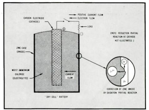
Figure 1. Illustration of electrochemical nature of corrosion – corrosion of zinc anode in dry cell battery.
