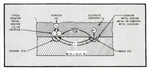
Figure 2. Illustration of electrochemical nature of corrosion – corrosion of single mental in contact with corrodent.
