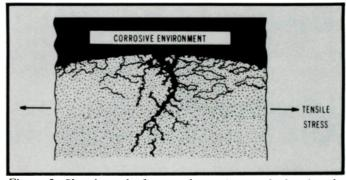
Figure 5. Sketch made from a photomicrograph showing the stress-corrosion cracking of a 2024-T351 aluminum alloy hose fitting loaded in hoop stress.
