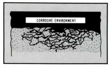
Figure 6. Sketch made from a photomicrograph showing intergranular corrosion in an aluminum alloy.
