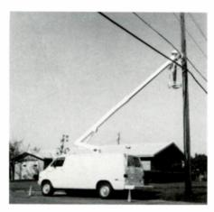
offers a working height of 30 feet, full 360° rotation and an elevation range of -6° to +84°. Rated bucket capacity is 300 pounds, and the VAN-TEL meets all OSHA standards without ballast, outriggers or stabilizers, even
