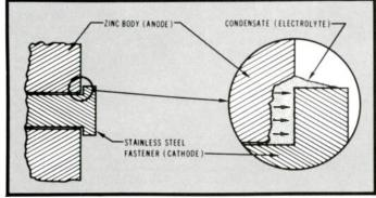
Figure 3B. One example of how galvanic corrosion could occur in practice,
