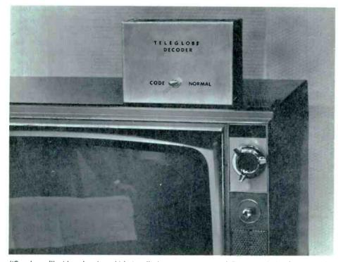
"On channel" video decoder which installs between antenna and TV set and signals scanner in same manner as Speaker Control Unit so that Centralized Metering and Billing is possible with this version of the system.
