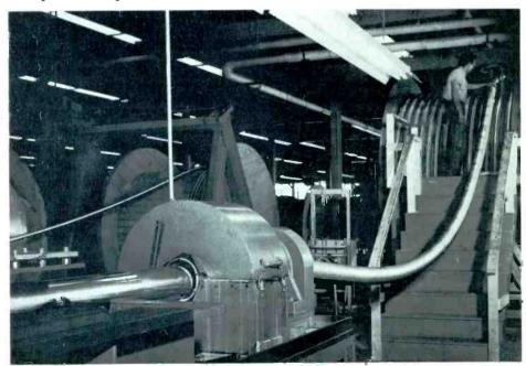
Last part of the forming process takes place when the machine shown here convolutes the outer conductor. Cable is then placed on a reel and tested.
