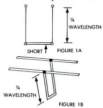
since the open-end has an impedance that is extremely high and for all practical purposes causes no effect when added. To carry this further, a series of these shorted, quarter-wavelength sections of line could be grouped about one spot with a result that would be the same as obtained with a single section except for reduced conductor resistance and higher "Q". Taking this example, Figure 2, a fundamental cavity is formed from this group. Closing in the sides completes the formation.
