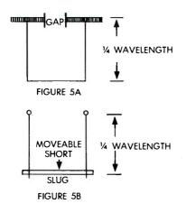
In most cases, the analysis of a cavity is applicable back to a simple section of transmission line. This includes such items as coupling to a cavity by probes or loops. Although this is an oversimplified method, it is easier to see and understand than talking about E and H fields, permittivity, permeability and flux density.
