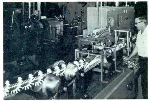
At this point on the production line the inner conductor with its polyethylene dielectric is being fed toward the welding machine while the outer conductor strip is rolled around the inner assembly and subsequently welded.
