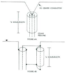
In Figure 4 two types of linear "baluns" are shown.
