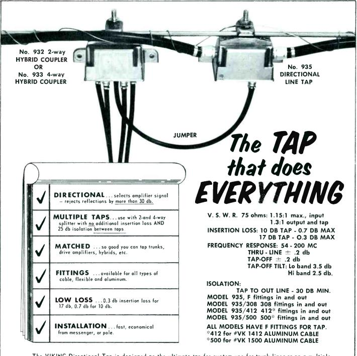
The VIKING Directional Tap is designed as the ultimate tap for system use for trunk lines or as a multiple tap source or as a bridging device.
