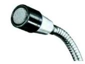
The unit is compact (2-41/64 inches long, 1-23/64 inches diameter), and is voice-response peaked for base station installations. The unit has a low impedance permitting unusually long cable runs without adverse affects on response characteristics or levels. Frequency response is 40 to 10,000 cycles with a rising characteristic to 4,500 c.p.s. Price on the new microphone is \$32.50.
