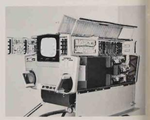
Plug-in transistorized modules speed servicing, increase reliability.
