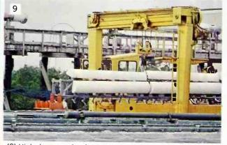
(9) High-rise crane truck, shown conveying special UHF Panel antenna to testing site, is typical of many special equipments employed in this unique antenna engineering site. Pylons in foreground await shipment.
