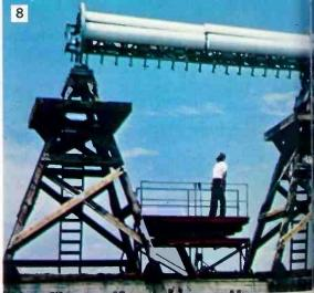
(8) Giant turntable called "Tiny Tim" where test antennas up to 15 tons move on a circular track 90 feet in diameter. It is one of three large turntables available for testing.
