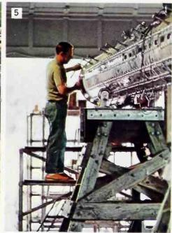
(5) Assembling one of the largest Pylon Antennas ever built. It will provide a base for a large Super Turnstile antenna in a stacked
