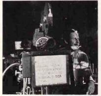
Tv camera mounted on right side of film camera is used as monitor.
