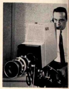
New RCA one-tube, low-cost camer may have application in testing idea for color commercials via CATV.
