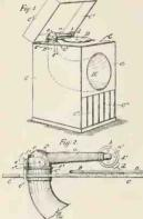
universal joint provided with means for holding the tubular arm and diaphragm box in raised position.
