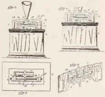
ment with the cylinder. Fig. 2 is a similar view but showing the position of the parts when the needle is out of engagement with the cylinder or during the shifting movement. Fig. 3 is a detailed perspective of the plate and its attachments. Fig. 4 is a plan view of the device.
